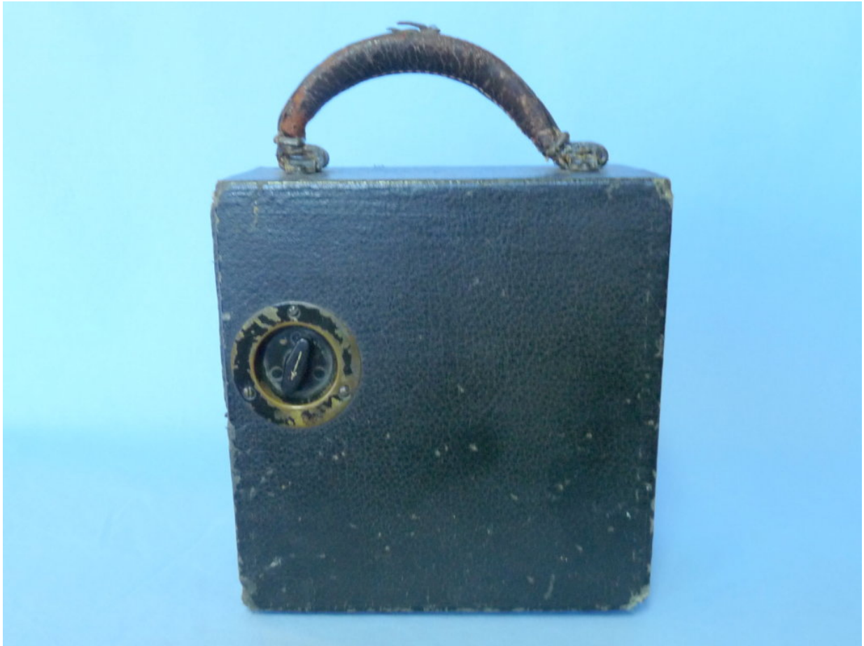
Figure 6. The back of the Vactuphone shows the volume control/on-off switch. This is the side that faced you so you could easily adjust the volume.
