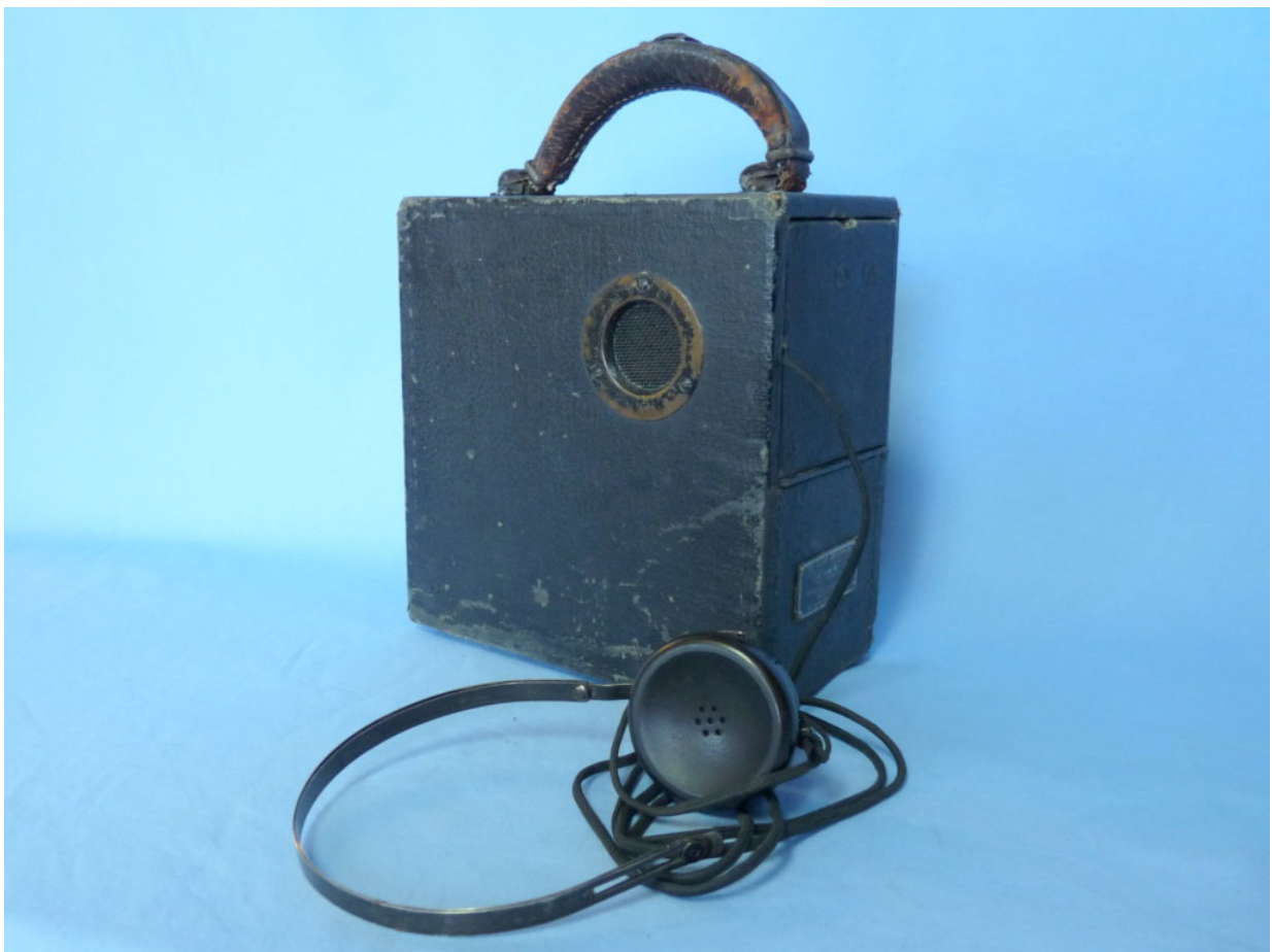
Figure 1. The Vactuphone vacuum-tube hearing aid of 1921—the world's first commercially available electronic hearing aid complete with single earphone on headband.
