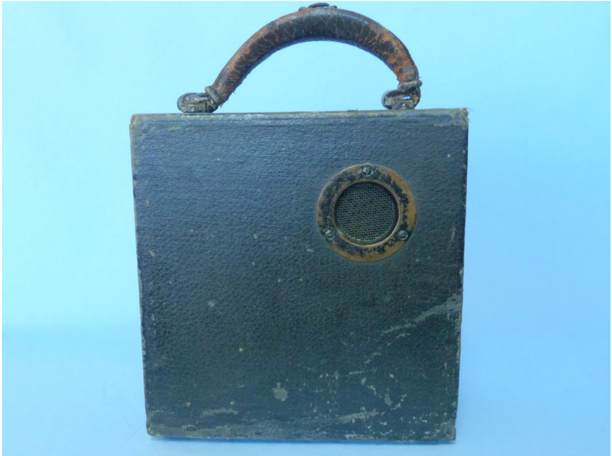
Figure 5. The front of the Vactuphone showing the microphone grill. This is what the person you were talking with saw.
