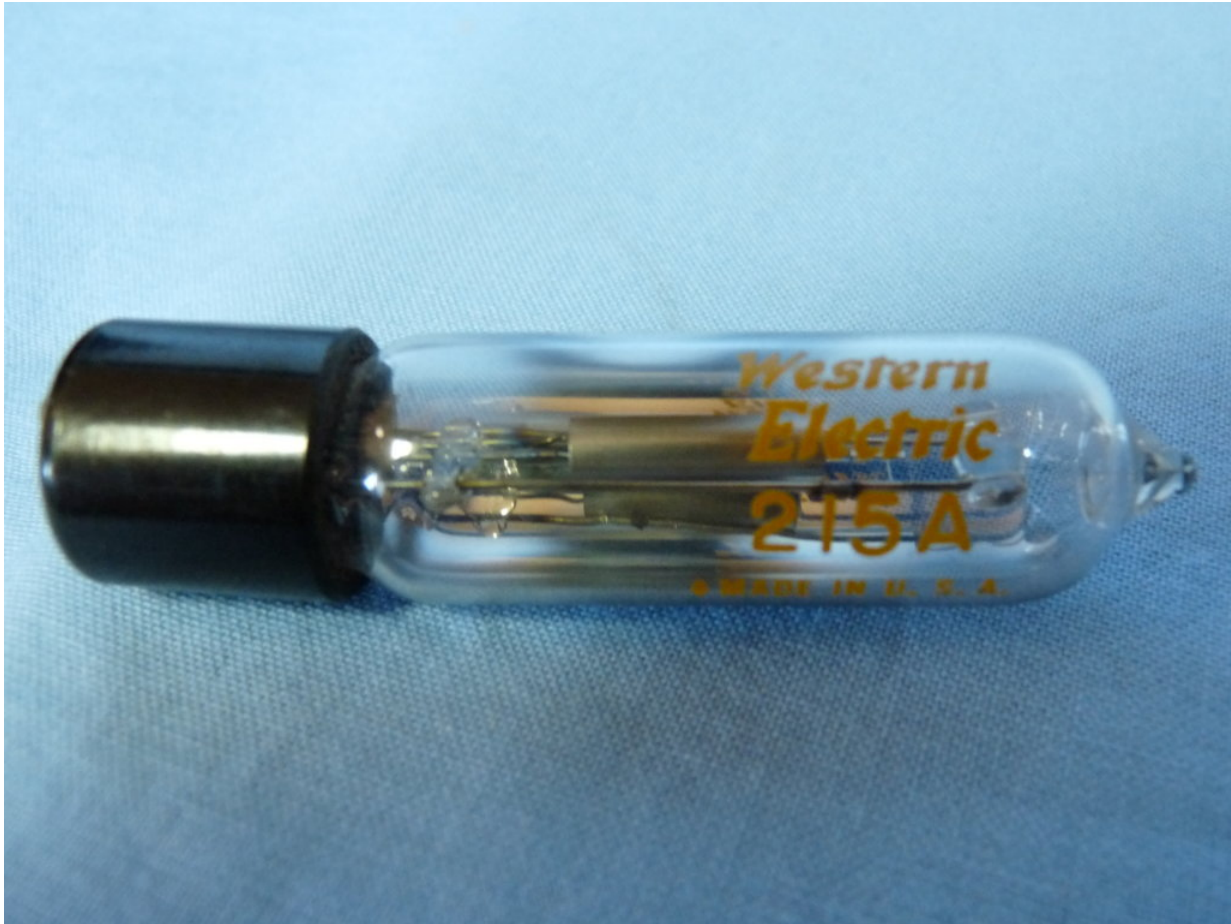
Figure 4. The heart of the Vactuphone was Western Electric's 215A triode "peanut" tube. It was 2 9/16" (6.5 cm) long and 5/8" (1.6 cm) in diameter.
