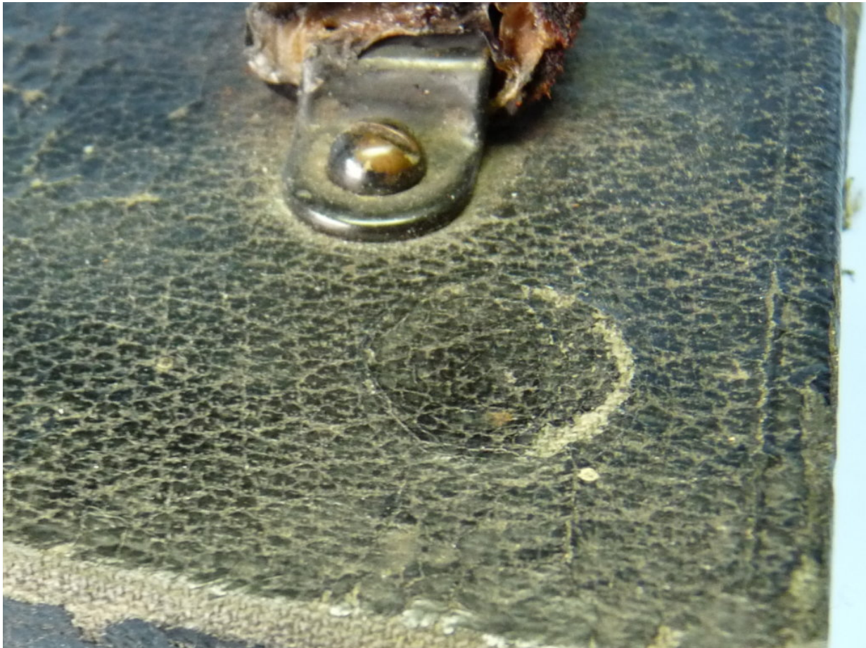
Figure 9. The hidden button to gain access to the electronics compartment. You can see the faint circle on the top right corner of the case where you pressed to release the hidden catch.
