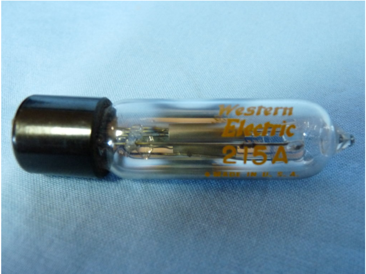
Figure 4. The heart of the Vactuphone was Western Electric's 215A triode "peanut" tube. It was 2\frac{9}{16} " (6.5 cm) long and \frac{5}{8} " (1.6 cm) in diameter.
