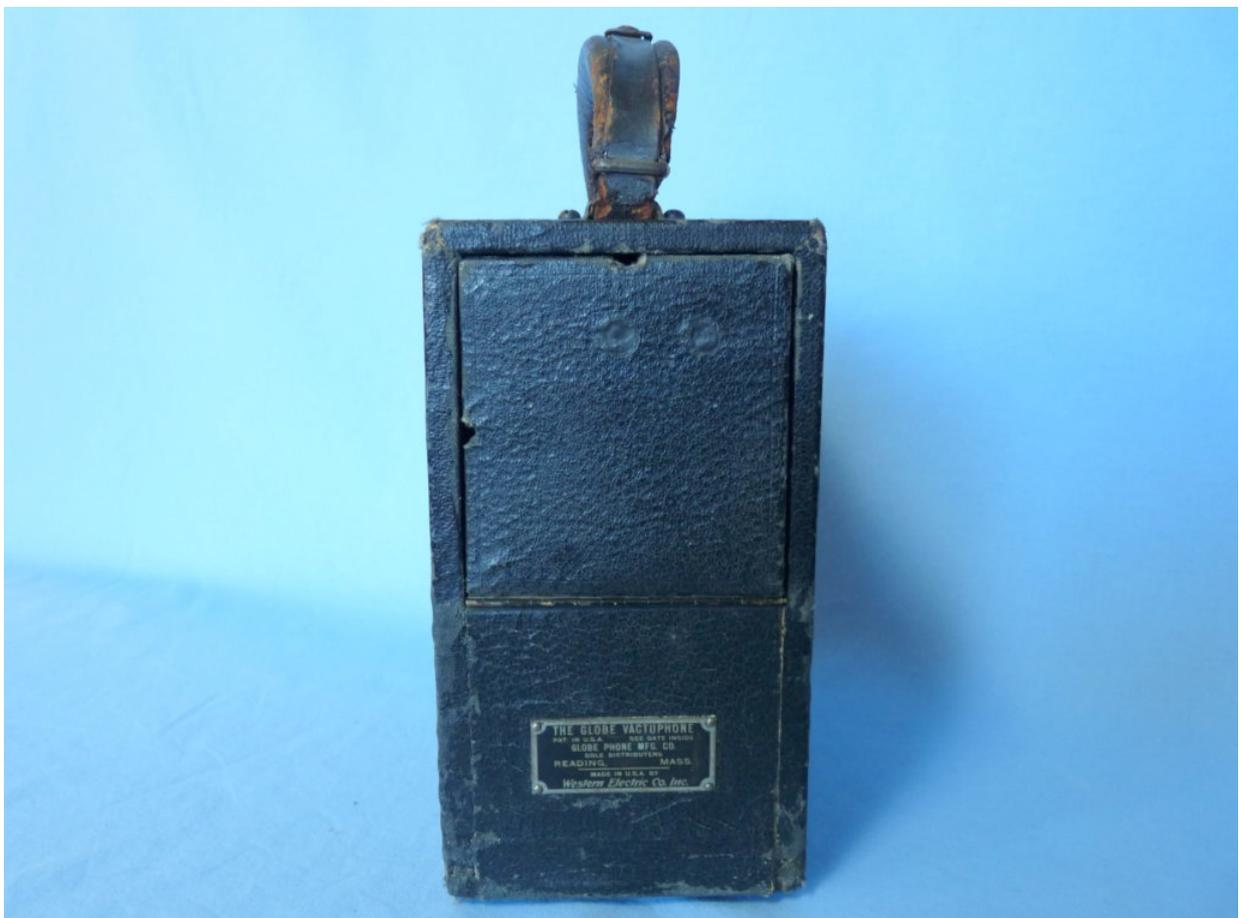
**Figure 8.** The right end of the Vactuphone shows the hidden trap door giving access to the electronics compartment (top half) and the nameplate (bottom). Note the two half-round holes on the top center and left center of the trap door. These were for the earphone cord to come through when using this hearing aid. You chose whichever hole you wanted depending whether you were standing up or sitting down.
