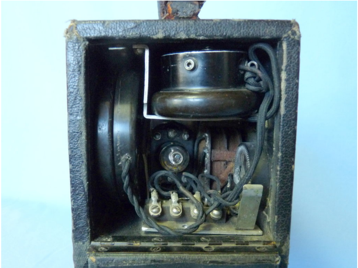
Figure 7. Inside the electronics compartment. The carbon shot microphone is on the left, the vacuum tube is dead center, and the volume control is on the right. In the top right is the storage compartment for the earphone and cord when not in use.
