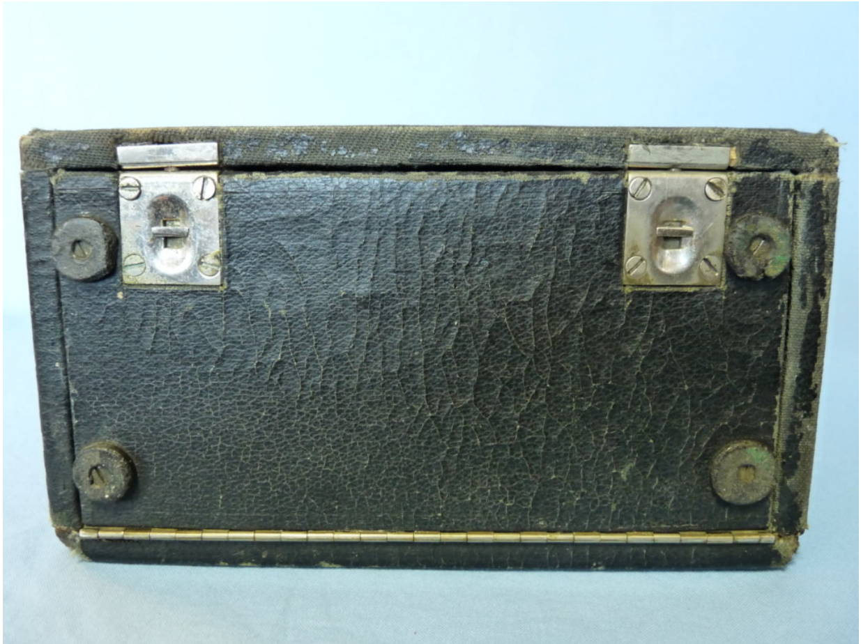
Figure 3. The bottom of the Vactuphone showing the door to the battery compartment.
