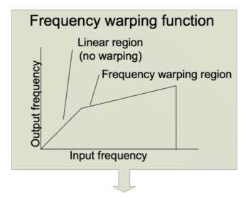
Frequency translation is applied according to a piecewise-linear warping function.
