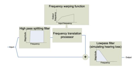
Figure 4. System Block diagram of Starkey Frequency-Lowering system.
