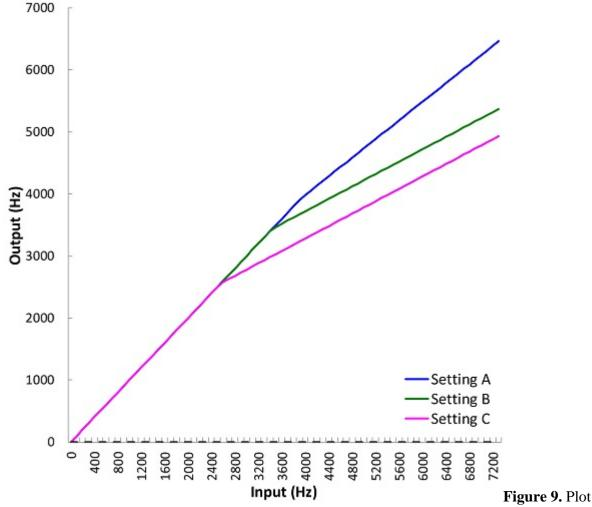
showing the frequency input-output functions for the three settings available in ReSound's Sound Shaper (different colors). Notice that compared to Figure 6, these lines have the appearance of 'broken-stick' functions (two lines, with different slopes) on a linear frequency scale. This is a byproduct of the 'proportional' compression discussed in the text. Source: Sound Shaper Fitting Assistant.
