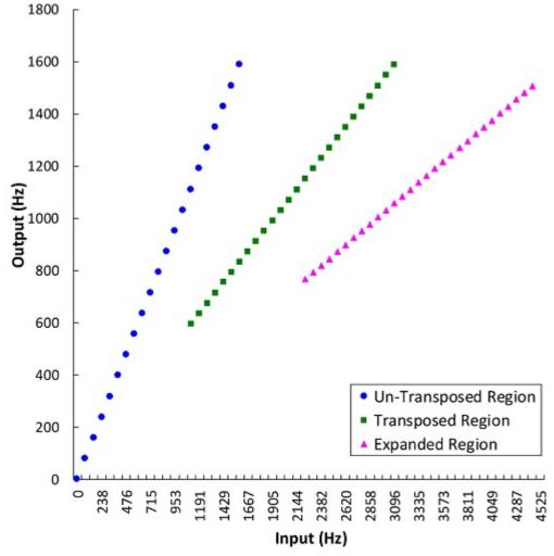
**Figure 1.** Plot showing how the frequencies at the input of the hearing aid are altered at the output by Widex's Audibility Extender. The un-transposed signal (blue circles) is low-pass filtered above the start frequency (1600 Hz in this example), but this frequency can now be optionally changed with the new Enhanced Audibility Extender. The transposed signal (green squares) overlaps with
