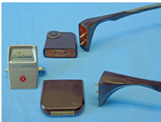
Figure 4. The Radioear Model 840 eyeglass hearing aid pulled apart to make a body-worn hearing aid. The aluminum face-plate (left) was sandwiched between the two parts.
