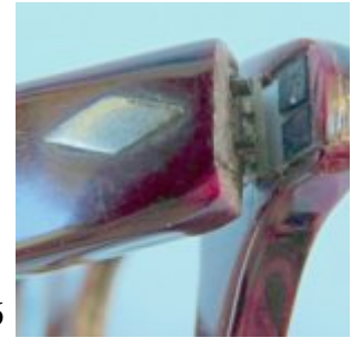
Figure 6. Close-up view of the hinge area of the Otariion Model L10 eyeglass hearing aid showing the black "pins" (left) and "plates" (right).
