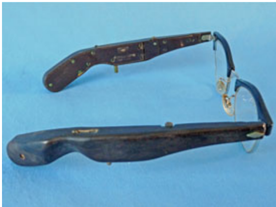
Figure 7. The Acousticon Model A-235 eyeglass hearing aid only required one temple-piece. This is an example of the first pieces – it's just that all the hearing aid to have a separate hearing aid in each temple-piece.
