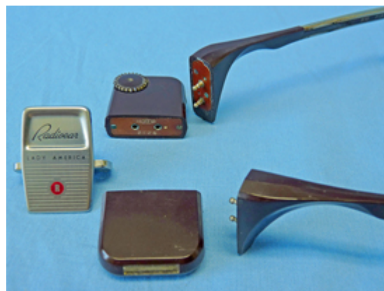
Figure 4. The Radioear Model 840 eyeglass hearing aid pulled apart to make a body-worn hearing aid. The aluminum face-plate (left) was sandwiched between the two parts.
