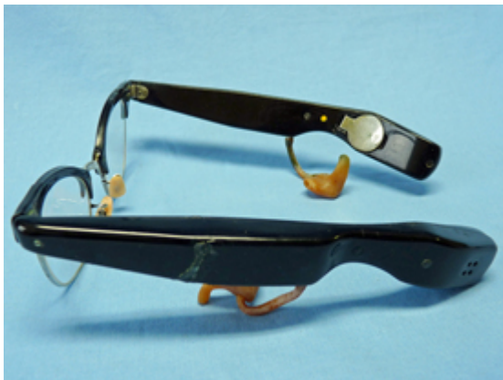
Figure 8. The Beltone Hear-N-See eyeglass hearing aid was another early hearing aid that only required one temple-piece. This example also had a separate hearing aid in each temple-piece – quite a rare occurrence back in the mid-1950s.
