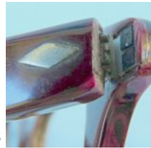
Figure 6. Close-up view of the hinge area of the Otariion Model L10 eyeglass hearing aid showing the black "pins" (left) and "plates" (right).
