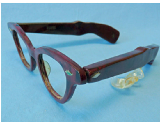
Figure 1. Otation Model L10 “Listener” eyeglass hearing aid—the world’s first transistorized eyeglass hearing aid. Note the thick, heavy temple-pieces. Both were needed for this hearing aid.
