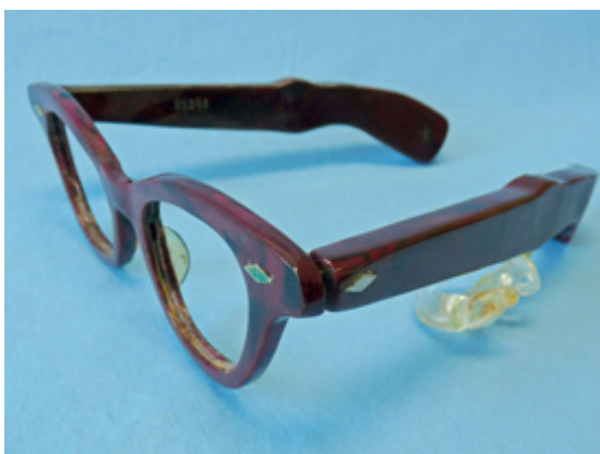
Figure 1. Otariion Model L10 “Listener” eyeglass hearing aid—the world’s first transistorized eyeglass hearing aid. Note the thick, heavy temple-pieces. Both were needed for this hearing aid.
