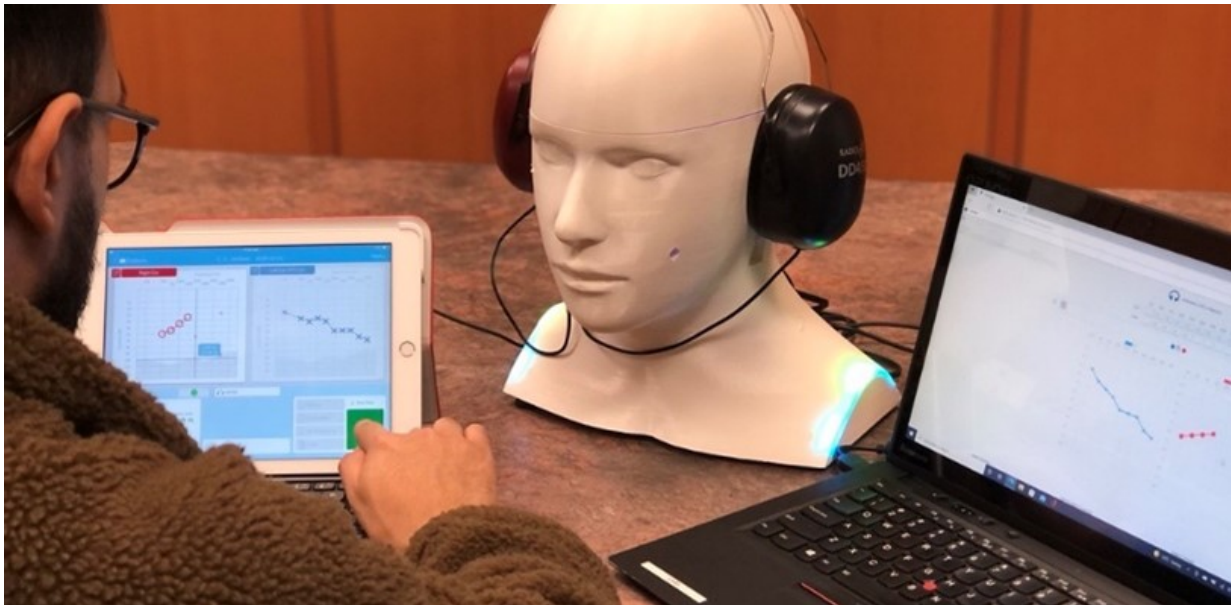
Figure 4. A prototype CARL manikin in use to simulate hearing loss for audiometry practice.
