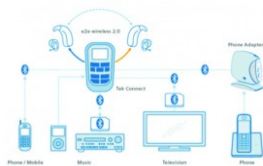
Figure 3. Connectivity options with e2e wireless 2.0 and Tek.
