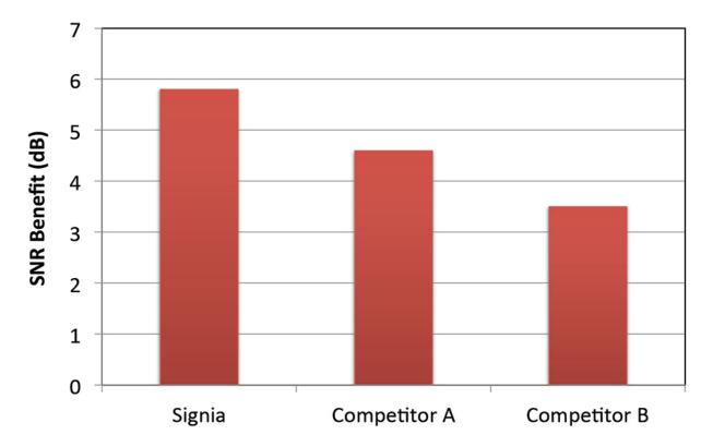
**Figure 2.** Signal-to-noise (SNR) benefit for the primax CROS for an adaptive speech test; transmitter microphone ON versus OFF. For comparison purposes, SNR benefit is also displayed for two competitor CROS models, taken from published research with these instruments.
