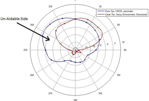
**Figure 1.** Ratio of interfering to target signal level at 1000Hz. Target is fixed at 0° while interferer direction is varied. Curves are given for transmitting and receiving side of the Signia BiCROS solution in noisy environments (receiver on right).
