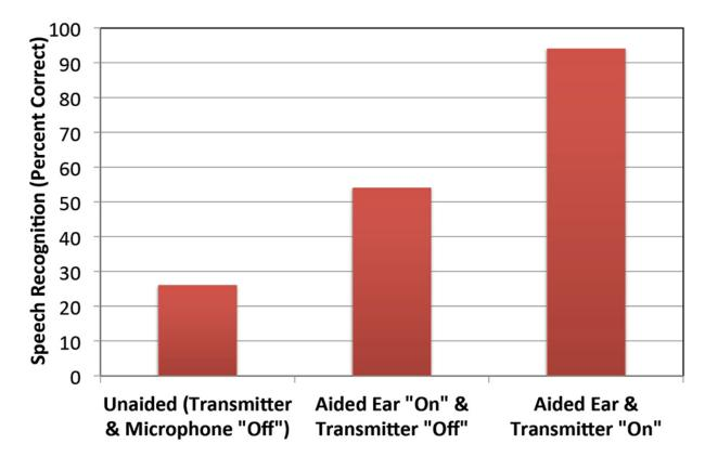
**Figure 3.** Mean speech recognition (percent correct) obtained for clinical testing of Signia primax BiCROS fittings for three settings: transmitter and receiver microphone off, receiver microphone on and transmitter microphone off, and both receiver microphone and transmitter microphone on.
