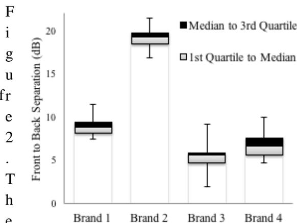
results of the directional microphone testing are shown. The front-to-back separation in decibels is shown for each brand. The whiskers indicate the range of the data.
