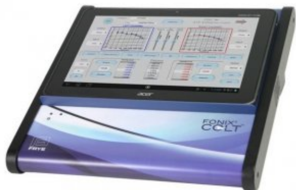
Figure 6. The Colt touch screen audiometer by Frye Electronics (U.S.), based on the Android tablet. The tablet is removable.
