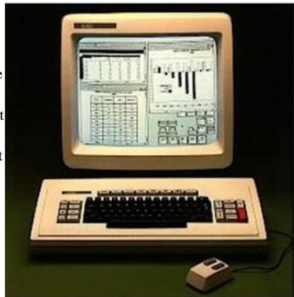
Figure 3. General GUI (Graphical User Interface) screen layout consisting of controls and readouts represented by numbers/graphs to fit the intended application, and accessed using a mouse.
