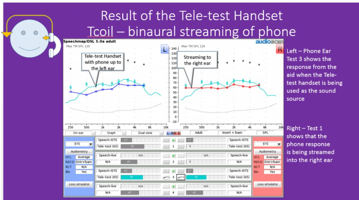
Figure 7. Binaural REM measure with tele-test handset (streaming).
