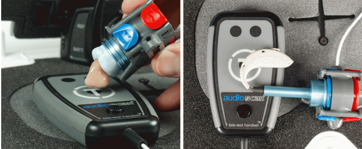
Figure 12. Hearing aid position for ANSI telecoil tests: Note that this test uses a 2cc coupler and specific hearing aid positioning.
