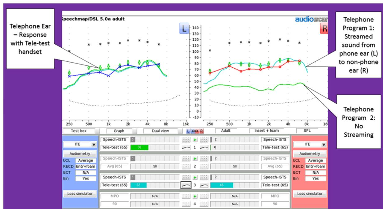
Figure 8: Tele-test measurement results with streamed (Test 1) and non-streamed (Test 2) telecoil program. In this example the hearing features were verified using SREM.
