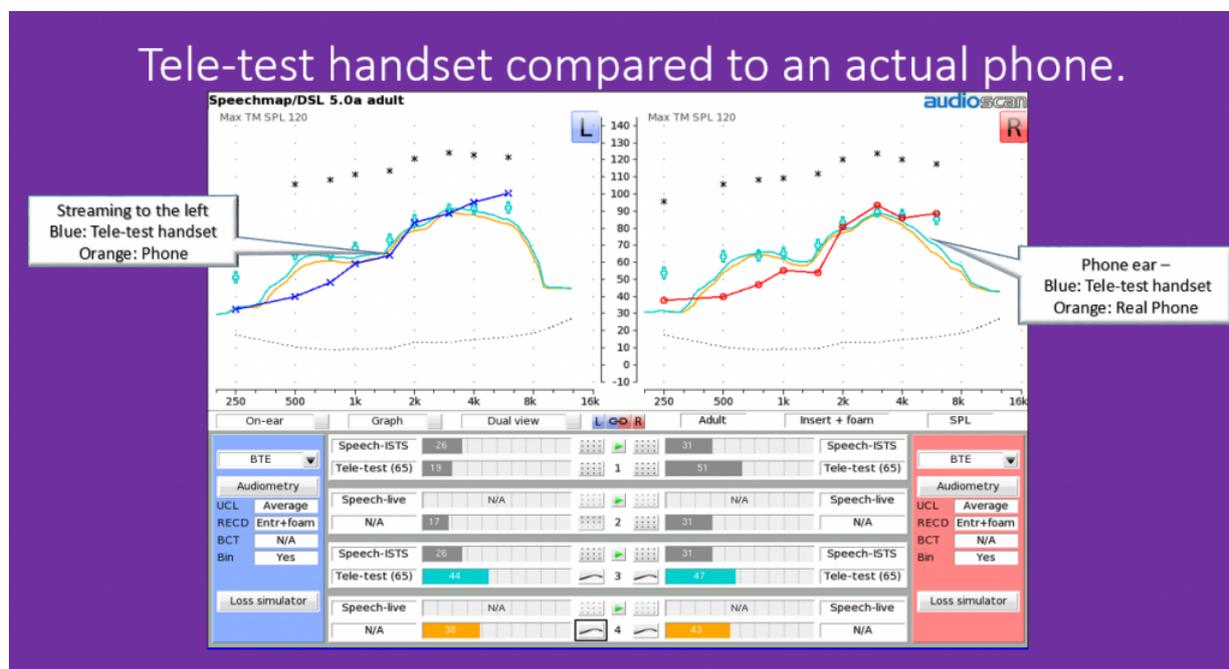
Figure 10. Tele-test handset compared to actual phone.
