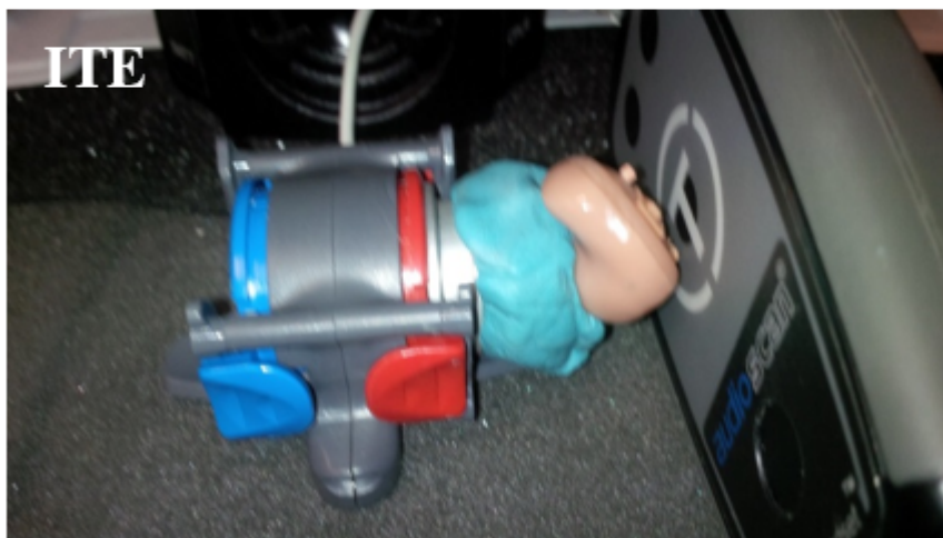
Figure 9. Coupler set up for BTE, ITE, RIC tele-test handset testing. Note the use of the magnet on the tele-test handset with the RIC. Its use allows for verification of autocoil function.
