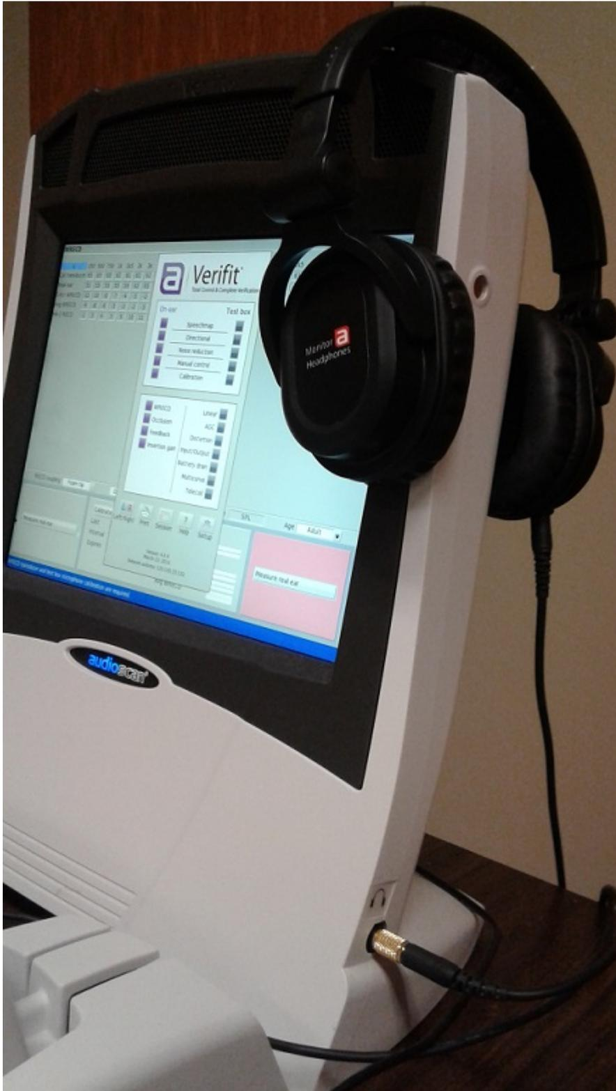
Figure 2. Monitor headphones of the VF2.
