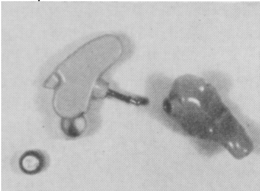
Figure 1. The original commercially-available auriculostomy hearing instrument, in a BTE format. It had a mini plug extending directly from
