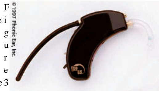
Phonic Ear Free Ear integrated FM receiver (courtesy of Phonic Ear).
