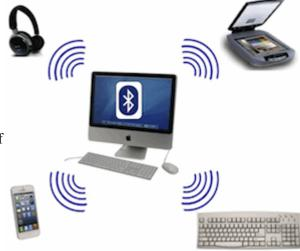
(10 meters or less) as would be needed for hearing Figure 1. Personal area network (PAN) set up aids. Up to eight devices can be connected, using Bluetooth technology. This shows a host
