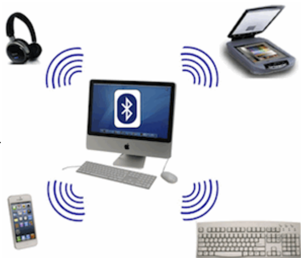
Figure 1. Personal area network (PAN) set up using Bluetooth technology. This shows a host
