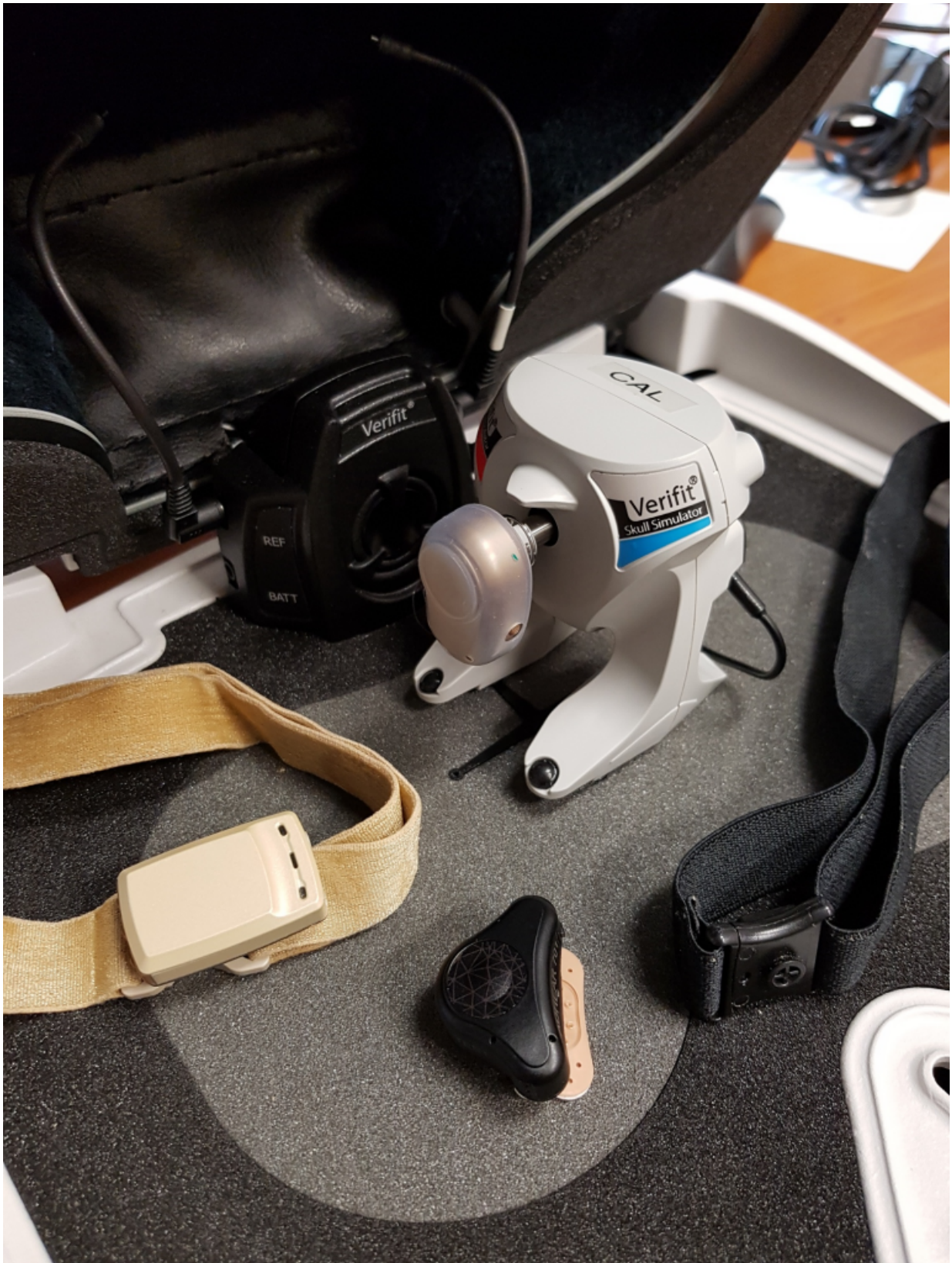
Figure 3. Various bone conduction hearing devices with soft headbands or adhesive strip. One device is attached to a skull simulator for verification.
