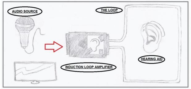
The diagram below shows a typical, complete hearing loop-to-hearing aid system.
