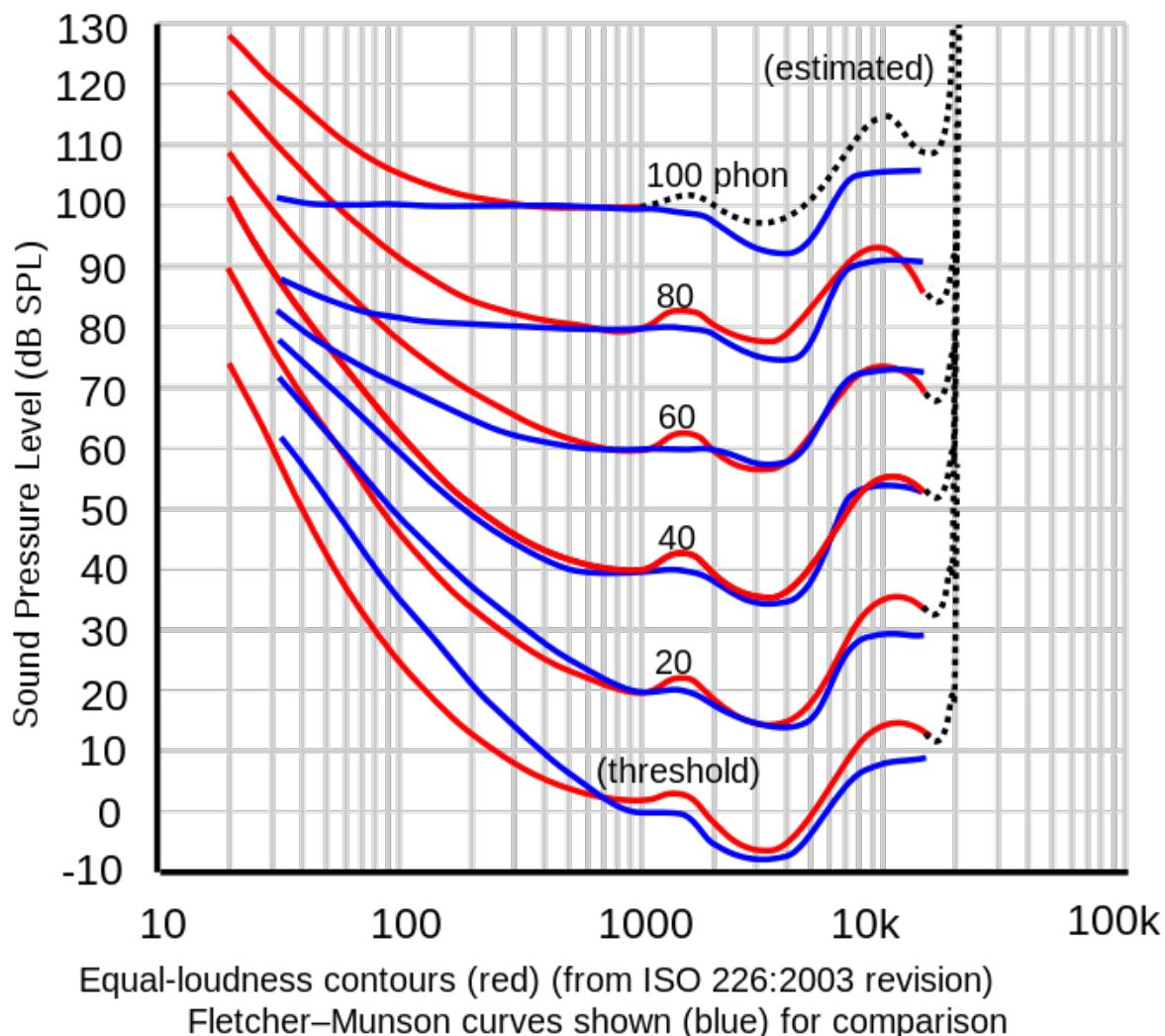
Our audiometers are calibrated following the threshold curves, meaning that when we set our instrument to present a tone under earphones of 0 dBHL at 1000 Hz, this is equivalent to saying that we are presenting a tone of 7 dB SPL. One could argue that this difference between dB HL and dB SPL is minimal at 1000 Hz, but if we go further down in frequency, for instance at 250 Hz, our audiometer is generating a sound pressure level of 25.5 dB SPL, and 45.5 dB SPL at 125 Hz.
