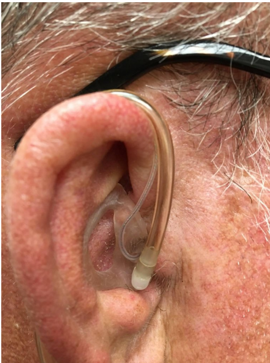
Figure 1. Earmold for both hearing aid and radio.
