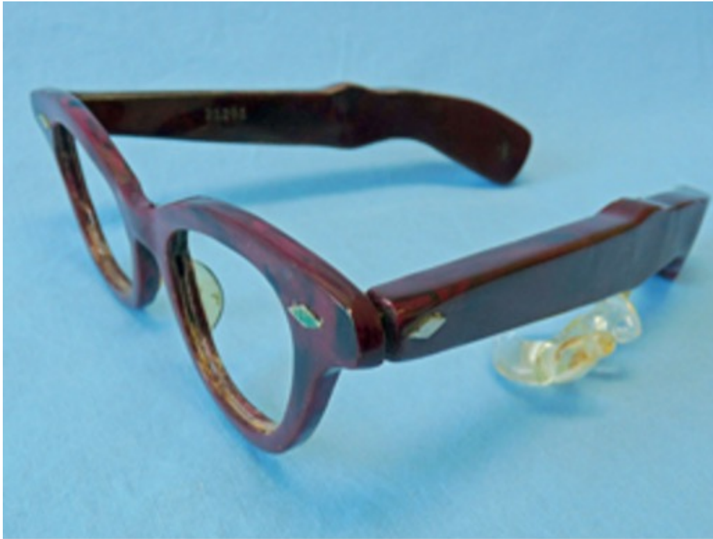
Figure 1. Otarion Model L10 "Listener" eyeglass hearing aid—the world's first transistorized eyeglass hearing aid. Note the thick, heavy temple-pieces. Both were needed for this hearing aid.
