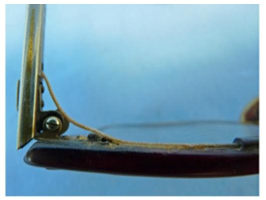
Figure 5. Radioear Model 840 eyeglass hearing aid showing how the wire threaded around the hinge and fitted into a groove along the top of the frames.
