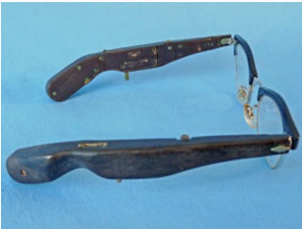
Figure 7. The Acousticon Model A-235 eyeglass hearing aid only required one temple-piece. This is an example of the first hearing aid to have a separate hearing aid in each temple-piece.
