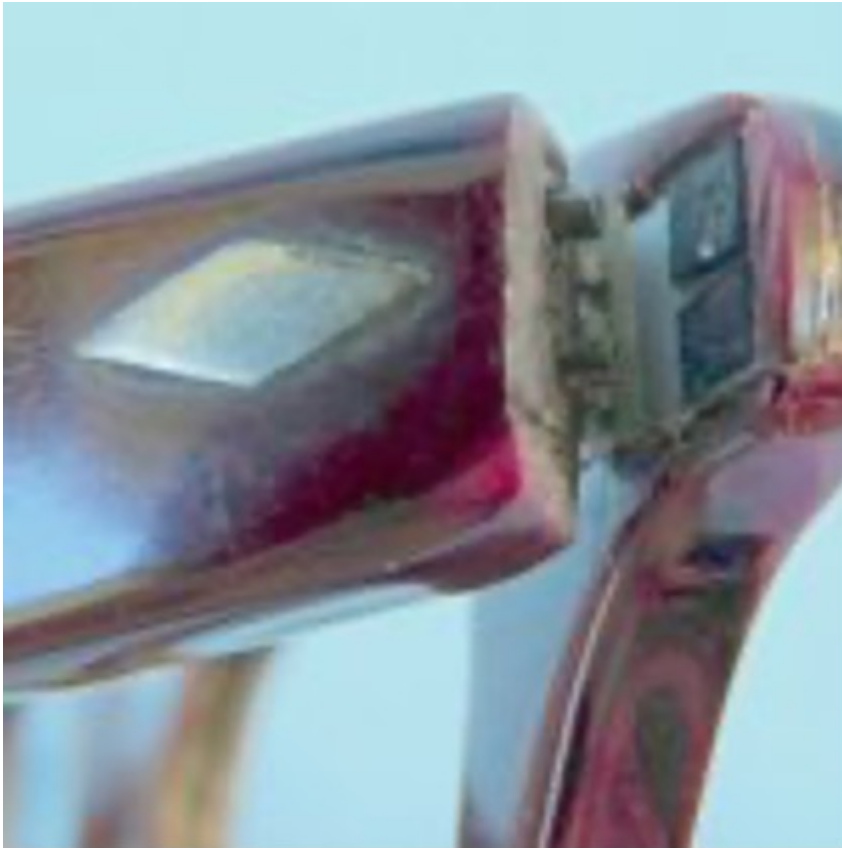
Figure 6. Close-up view of the hinge area of the Otation Model L10 eyeglass hearing aid showing the black "pins" (left) and "plates" (right).
