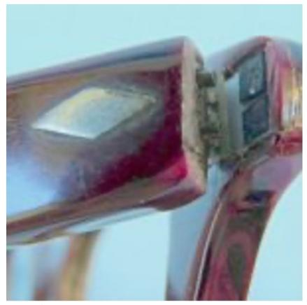
Figure 6. Close-up view of the hinge area of the Otarion Model L10 eyeglass hearing aid showing the black "pins" (left) and "plates" (right).
