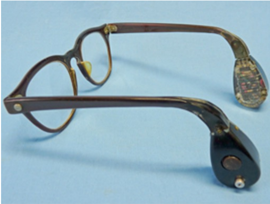
Figure 2. The Acousticon Model A-230 eyeglass hearing aid showing how the electronics were all contained in the tips of the temple-pieces.
