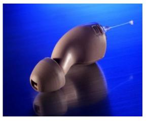
The instrument was designed for mild and moderate hearing losss. The goal was to develop a hearing aid that would overcome many of the hurdles causing many hearing impaired to delay wearing amplification and allow this with minimal involvement for entry into the system. The disposable hearing aid was intended to overcome consumer concerns related to:
