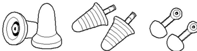
**Figure 2. Examples of push-to-fit earplugs.**
