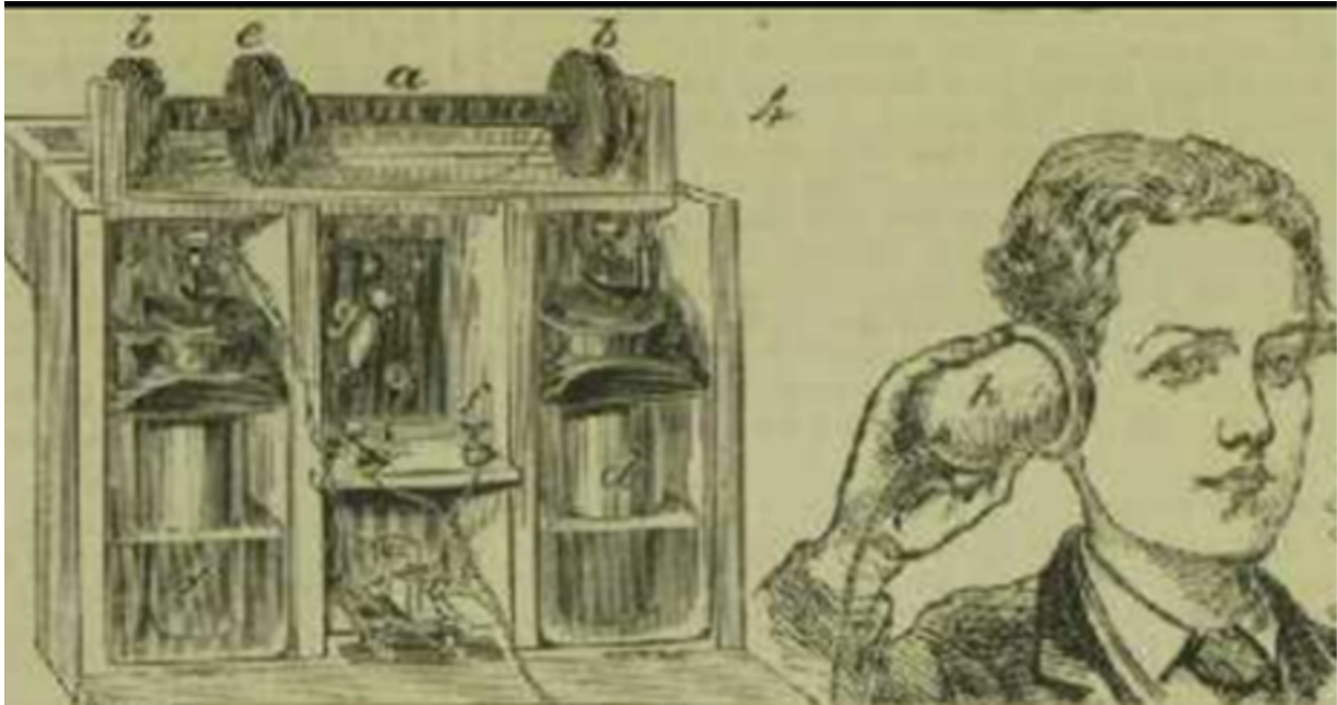
Figure 5. The Hughes audiometer (adapted from Illustrated London News 28 )
