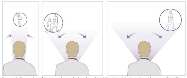
Figure 4. Examples of three settings of a hearing aid with adjustable directional beam widths. From left to right shows Narrow, Medium, and Wide correspond to listening scopes of approximately 50°, 70°, and 90° degrees, respectively.
