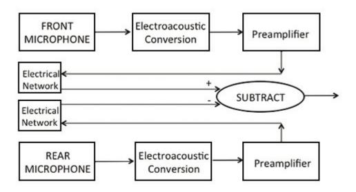
Figure 1. A schematic of how first-order directionality is achieved using two microphones in a digital hearing aid signal processor (adapted from Thompson<sup>5</sup>). By subtracting the electroacoustically converted and amplified signals from the front and back microphones, directivity patterns as shown in Figure 2 are created. When an omnidirectional response is required (ie, the majority of the time), the rear
