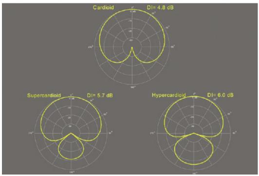
Figure 2. Examples of common directional polar patterns.
