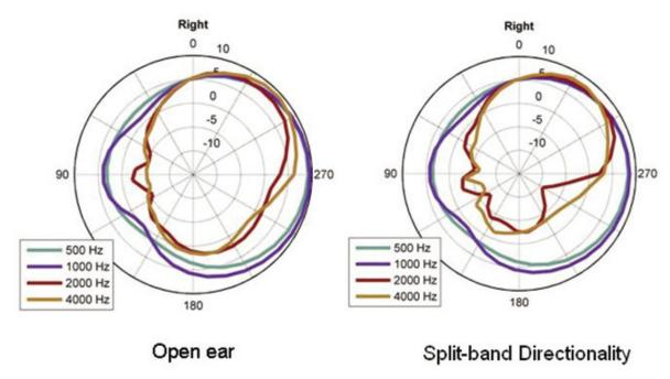
Figure 3. Directional responses of the open ear on the left and split-band directionality on the right. Note that the two lower frequencies are more omnidirectional while the two higher frequencies are heard more directional with attenuation to the sides and back.
