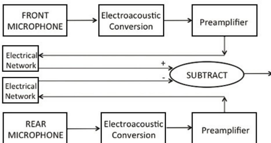
Figure 1. A schematic of how first-order directionality is achieved using two microphones in a digital hearing aid signal processor (adapted from Thompson<sup>5</sup>). By subtracting the electroacoustically converted and amplified signals from the front and back microphones, directivity patterns as shown in Figure 2 are created. When an omnidirectional response is required (ie, the majority of the time), the rear
