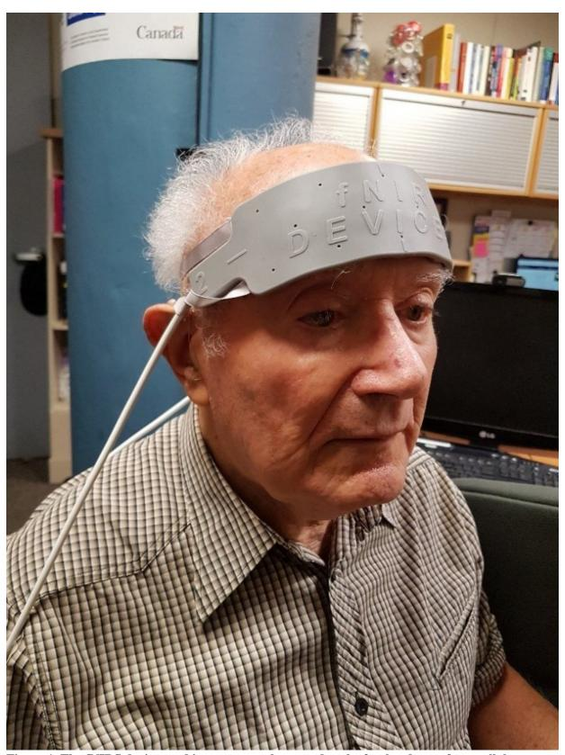
Figure 1. The fNIRS device used in our research secured to the forehead one of our collaborators,
