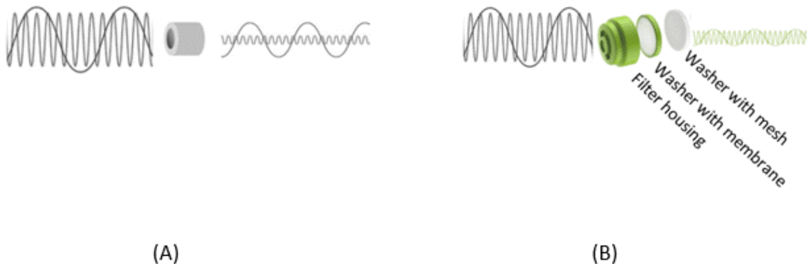
Figure 1: (A) – Traditional resistive tube filter which attenuates mostly high frequencies and (B) – Phonak Serenity Choice mesh and membrane filters.
