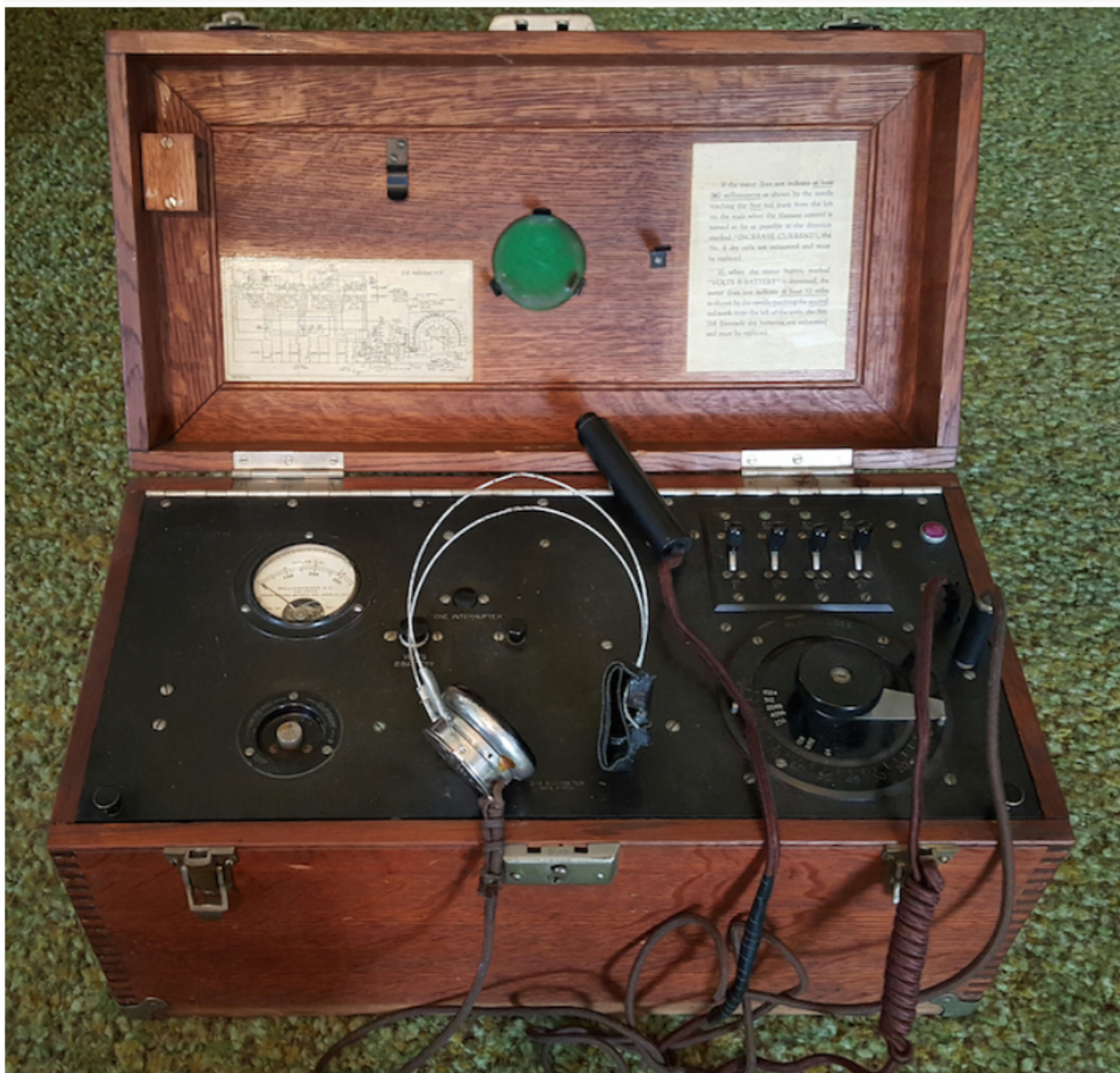
Figure 4. Western Electric 2-A audiometer.
