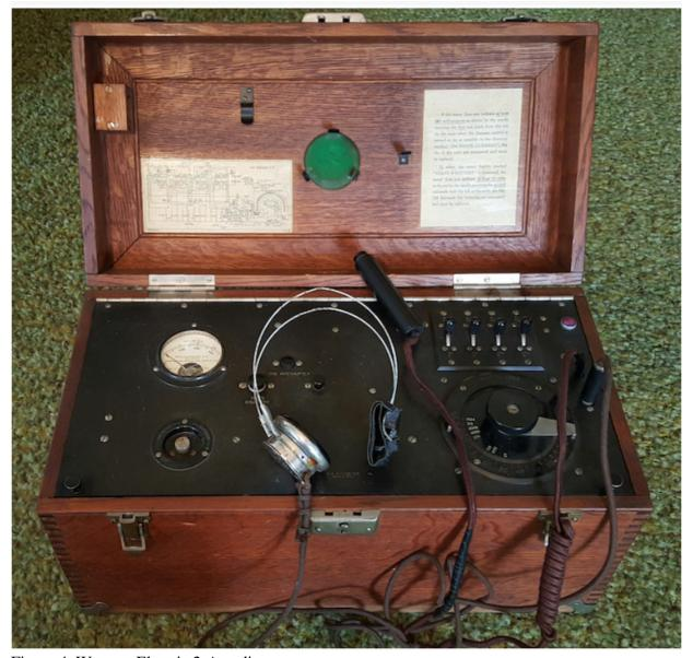
Figure 4. Western Electric 2-A audiometer.
