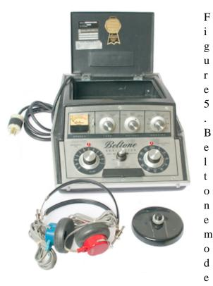
1 12D audiometer. Audiometers similar to this by Beltone and other manufacturers were commonly used in the late 1960s and 1970s.
