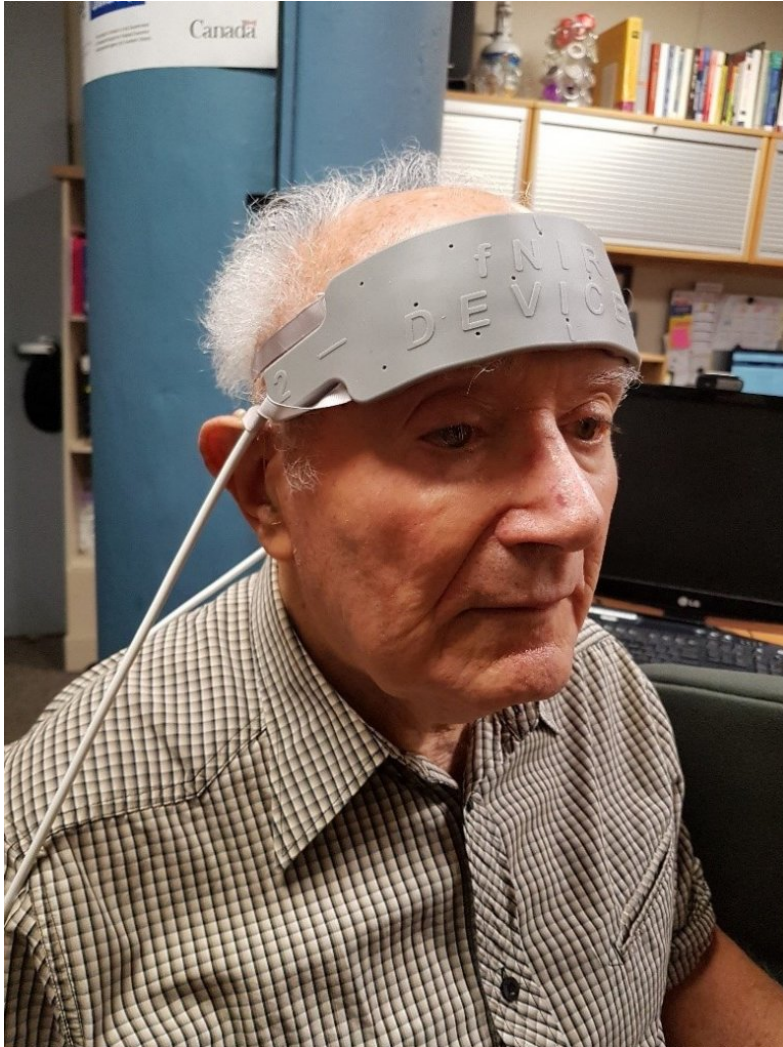
Figure 1. The fNIRS device used in our research secured to the forehead one of our collaborators, Alberto Behar. This device shines near-infrared light into the head over the PFC, allowing us to measure its activity.
