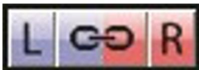
The BSFA tool is on by default in Verifit2 software versions 4.4 and later. To run tests simultaneously, select the L-R Link button on the Speechmap screen.
