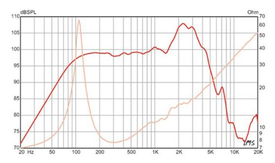
Figure 4. The frequency response (red line) plotted against the actual impedance (peach line) of the Eminence Red White and Blues guitar speaker.
