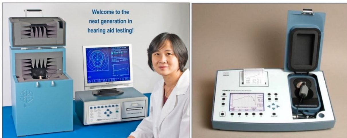
Figure 1. Hearing aid analyzers. Factory/Research model 8000 on the left, and office model FP35 on the right. Both instruments are capable of real-ear measurements as well. (Images courtesy of Frye Electronics).
