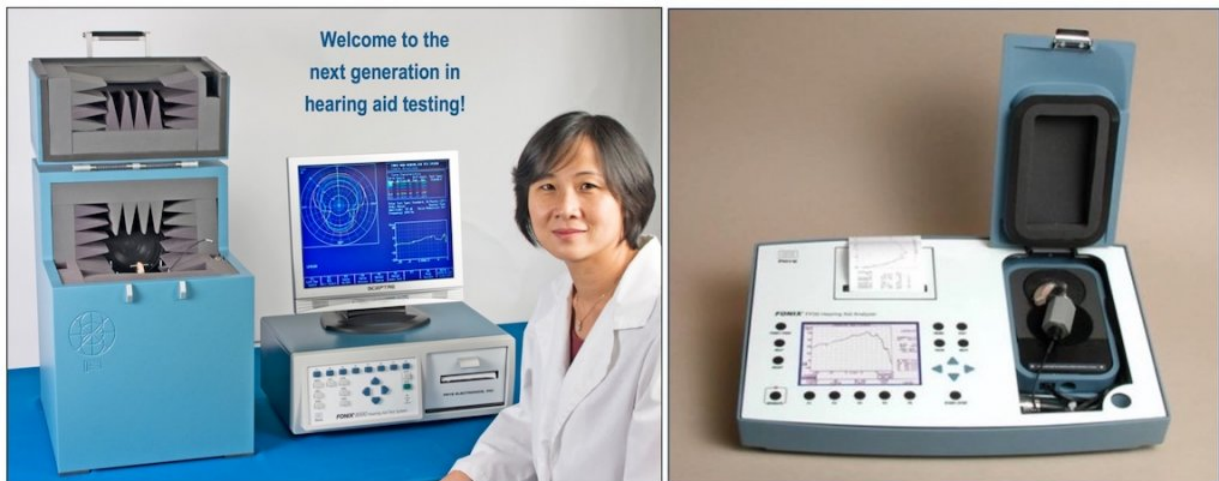
Figure 1. Hearing aid analyzers. Factory/Research model 8000 on the left, and office model FP35 on the right. Both instruments are capable of real-ear measurements as well. (Images courtesy of Frye Electronics).
