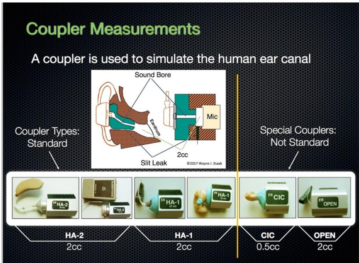
Figure 4. Measurement coupler configurations for hearing aids.
