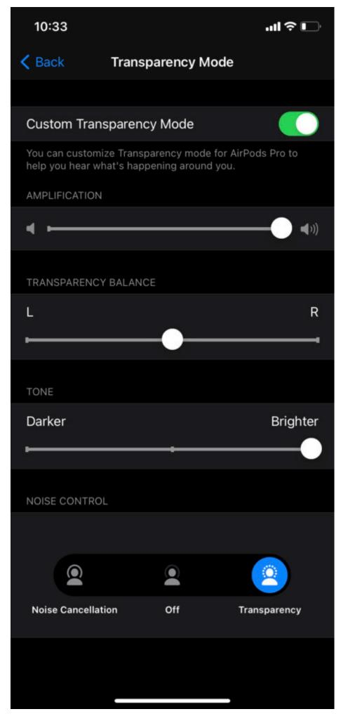
Figure 2. Transparency Mode on Apple's AirPods Pro enables the user to amplify live sound and customize the sound either via presets, a set of A/B comparisons, or the use of an audiogram.
