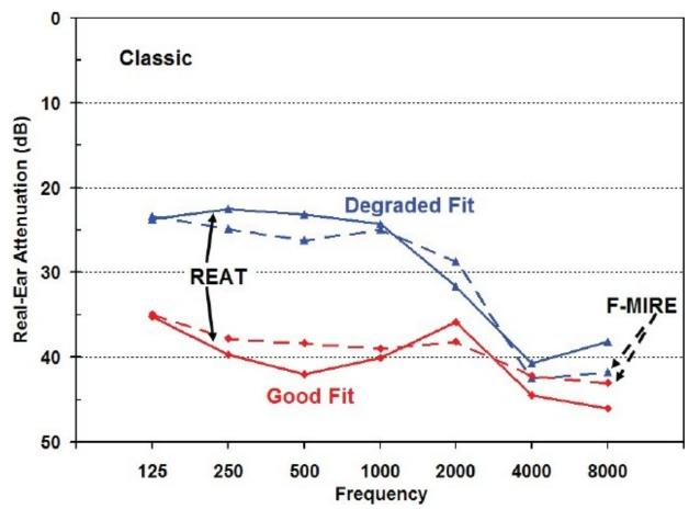
The NRR calculation is specified by the EPA's law, not the ANSI S3.19 standard. The NRR is computed from the mean attenuations and standard deviations of the attenuations for each of the nine (9) narrow bands of noise. The NRR is intended to predict the minimum amount of protection provided to 98% of potential users.
