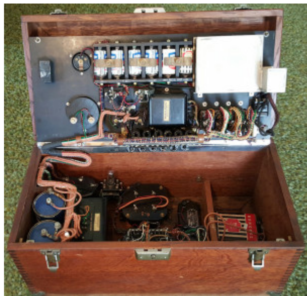
Figure 5. Electronics of the Western Electric 2-A Audiometer, with the plate raised.
