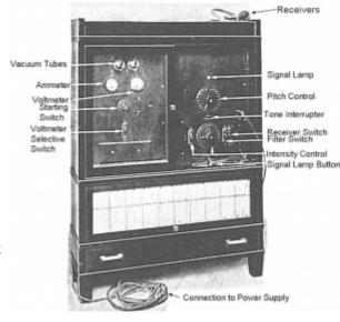
frequencies at octave intervals between 64 Hz and Figure 1. Western Electric 1-A audiometer. 8,192 Hz. The intensity range was limited, and an additional booster amplifier was needed to determine the threshold of feeling.
