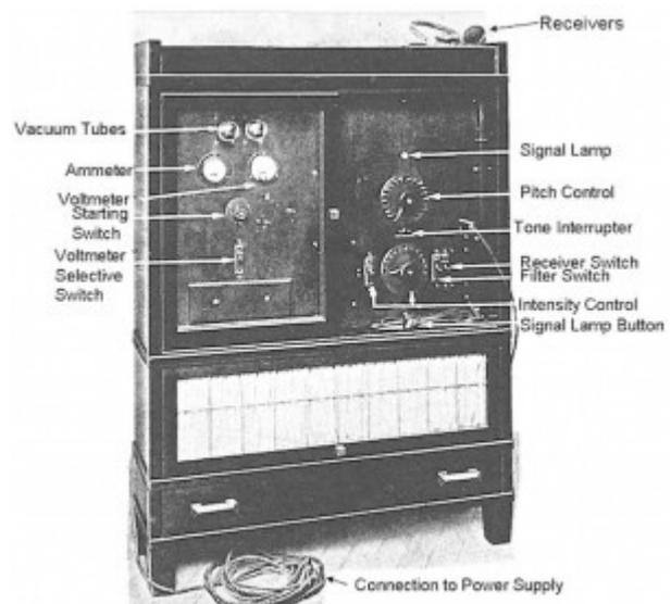
frequencies at octave intervals between 64 Hz and 8,192 Hz. The intensity range was limited, and an additional booster amplifier was needed to determine the threshold of feeling.
