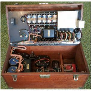
Figure 5. Electronics of the Western Electric 2-A Audiometer, with the plate raised.
