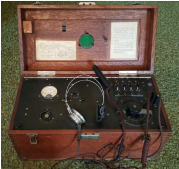
Figure 2. The Western Electric 2-A Audiometer.
