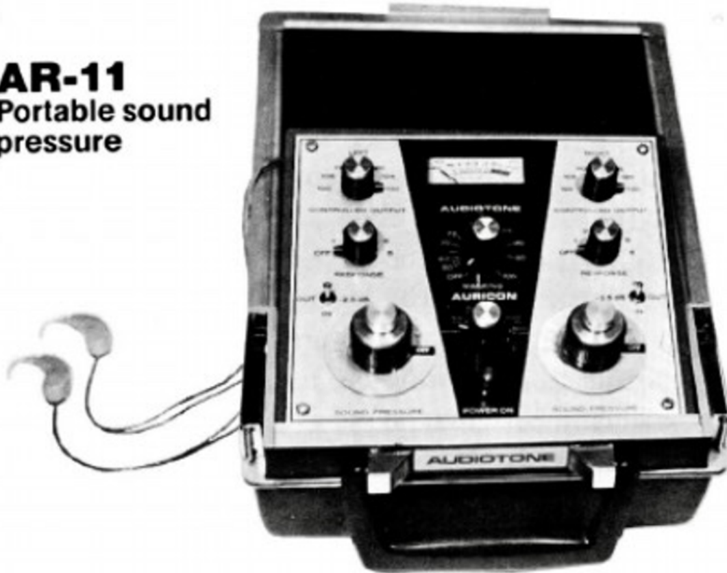
Figure 4. Shows the Audiotone Auricon, an assistive fitting device of the 1960s-1970s. It featured six graduated response options that could be installed in the selected hearing aid. For further information on master hearing aids, see Curran and Galster, 2013.1
