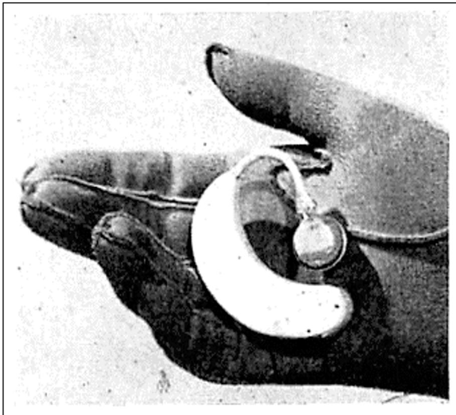
**Figure 2. The Zenith *Diplomat*, an early behind-the-ear instrument introduced in 1956. It featured a hand-wired 4-transistor amplifier and external body type receiver. Internal ear level receivers did not appear until 1959-1960.**
