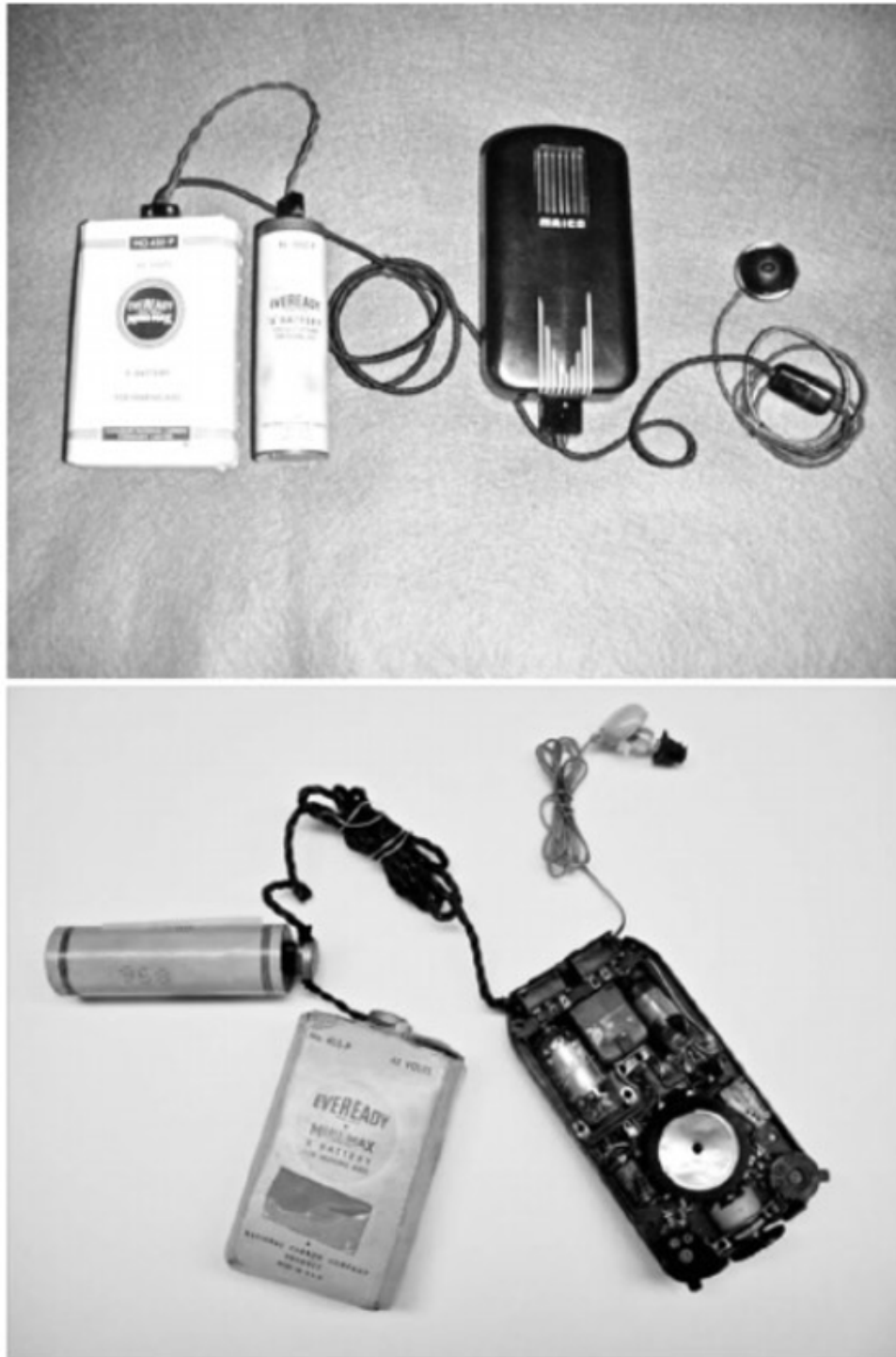
Figure 1. Two examples of 1940's era body-worn vacuum-tube hearing aids. The hearing aid, the two batteries and the receiver were worn externally.
