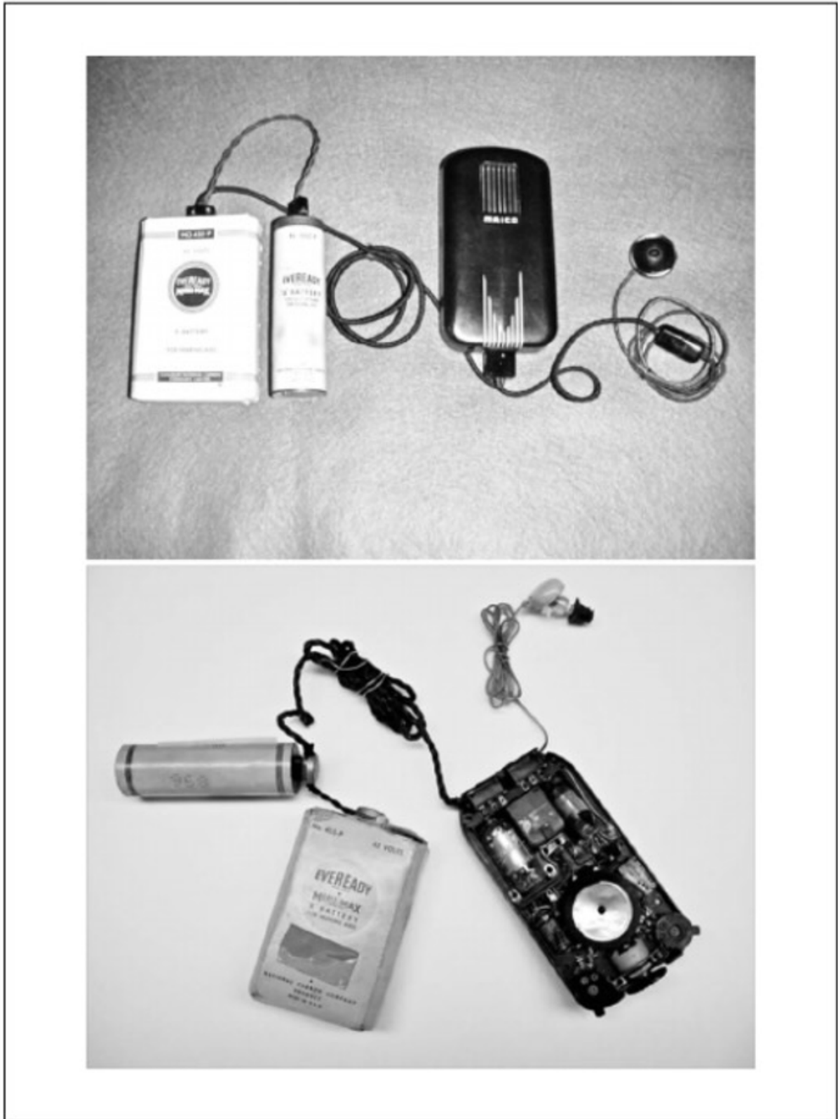
Figure 1. Two examples of 1940's era body-worn vacuum-tube hearing aids. The hearing aid, the two batteries and the receiver were worn externally.
