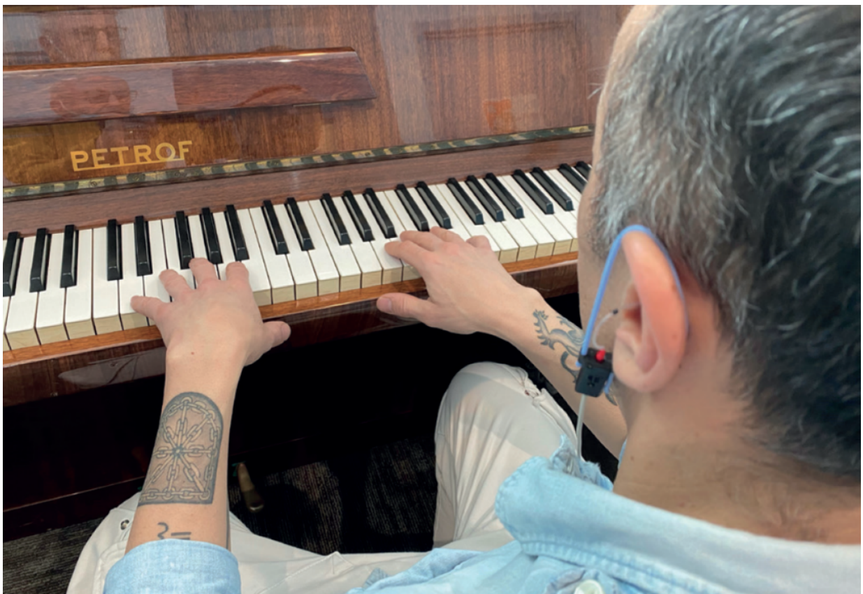
Real ear measurement can be performed while the musician is playing their instrument in order to provide precise sound level measurements with and without any specific hearing protection.
