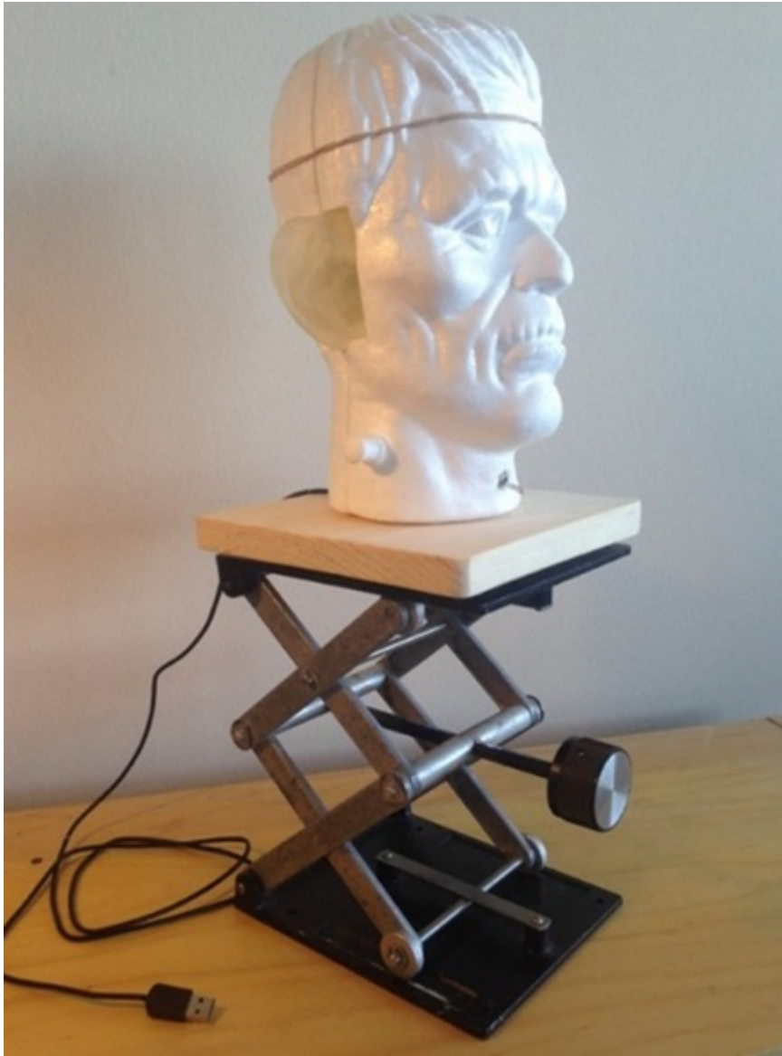
Figure 1. Early version of the Manikin-based probe-tube placement simulator.
