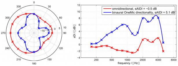
Figure 6. Polar pattern (ITR) for one-microphone binaural directionality at f=1kHz fitted to the left ear of the KEMAR (left panel). The sequential directivity index (sDI) is shown in the right panel.
