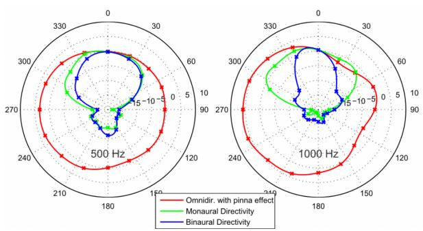
Figure 2. Polar patterns as measured with mini-BTE RIC (Pure carat 7bx) devices for f=500Hz (left) and f=1000Hz (right). The ITR is represented as the radial component in decibels, the angular components are the direction of arrival in degrees, where 0° is the frontal direction and 90° is the right side.
