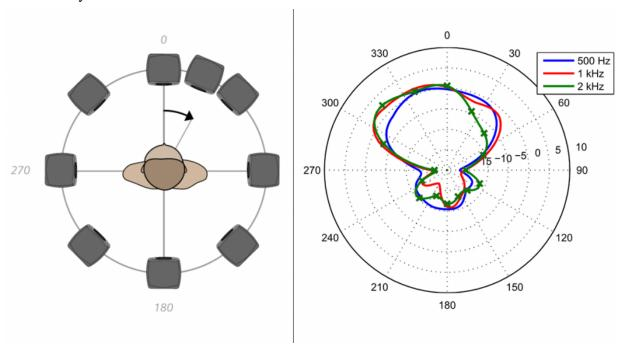
Figure 1: Left panel: Measurement setup. The KEMAR is rotated 22.5 degrees for the second round of testing. For more details about the approach, please refer to Aubreville and Petrausch7. Right panel: Interferer to Target Ratio (ITR) for standard directionality at three different frequencies.
