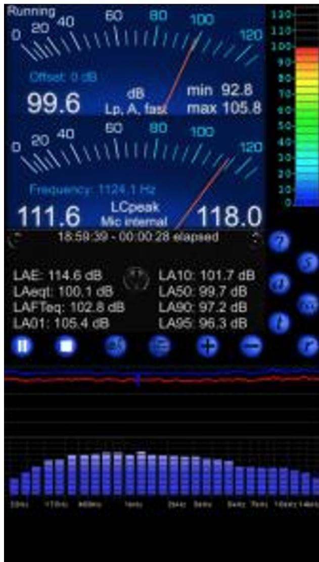
Figure 2. Sound level meter reading of the hand-dryer.
