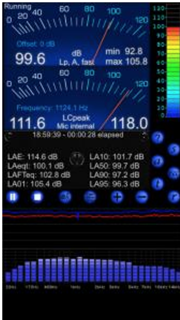
Figure 2. Sound level meter reading of the hand-dryer.
