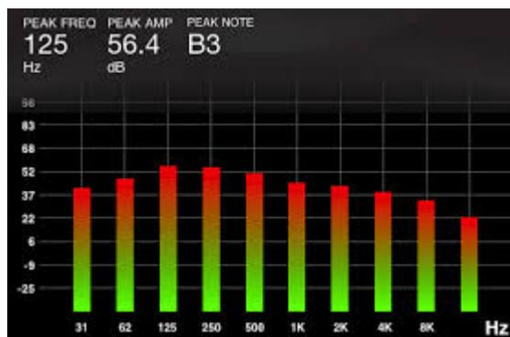
Figure 1. Octave band spectrum of a noise.
