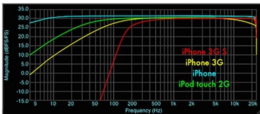
Figure 2. Input frequency response of various iPhone models, indicating high-pass filtering<sup>[6]</sup>.
