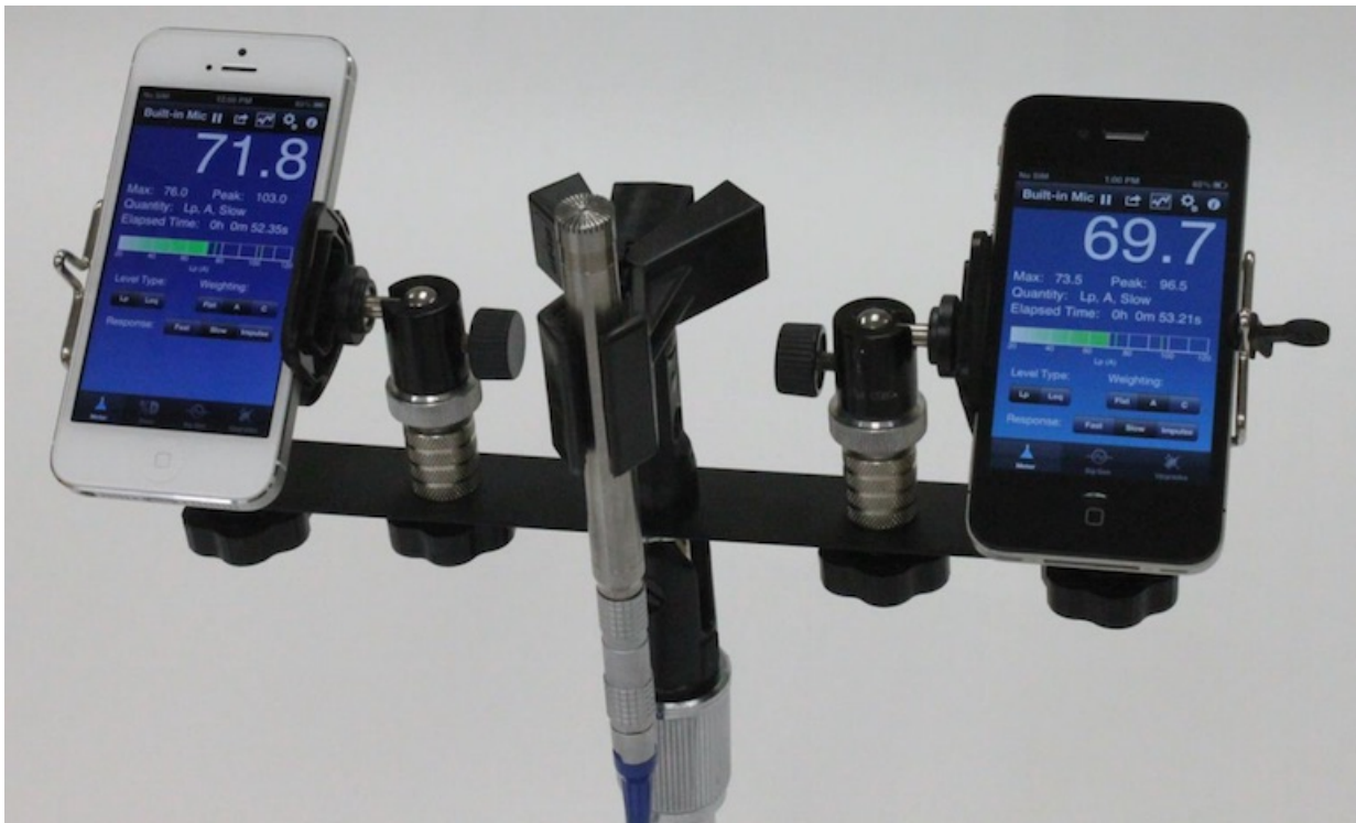
Figure 3. A suggested procedure for measuring and comparing smart phone sound level meter (SLM) apps. The SoundMeter app on the iPhone 5 (left) and iPhone 4S (right) compared to 1/2" Larson-Davis 2559 random incidence type 1 microphone (center). From Kardous and Shaw, (2014). The smartphones were attached to a stand in the middle of the reverberant sound chamber at a height of 4 feet, and about 6 inches from the reference microphone.
