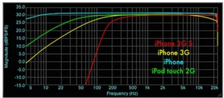
Figure 2. Input frequency response of various iPhone models,
