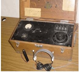
The first widely-used audiometer was the Western Electric 2A audiometer (1923). It ran on dry cells and was designed to meet clinical needs. In the early instruments, normal threshold values for each test frequency had to be established first to provide a reference. The instrument was limited to 8 frequencies at octave intervals between 64 Hz and 8,192 Hz. The intensity range was limited, and an additional booster amplifier was needed to determine the threshold of feeling.
