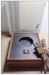
Figure 1. Miracle Ear Charger, hearing aid(s) turned off, but are left in the hearing aid with both placed in the round cavity. ensure adequate charge. (Staab collection, product of the late 1960s or early 1970s).
