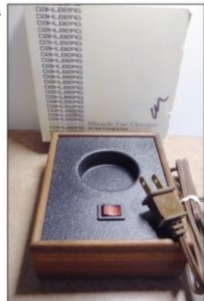
Figure 1. Miracle Ear Charger, Dahlberg Electronics, Inc., Hearing Systems Division. The hearing aid(s) turned off, but are left in the hearing aid with both placed in the round cavity. Batteries were to be charged daily for 8 hours minimum to ensure adequate charge. (Staab collection, product of the late 1960s or early 1970s).
