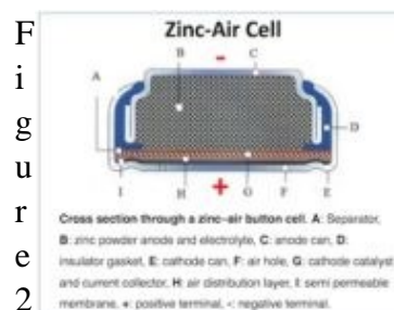
Zinc-air hearing aid battery diagram.
