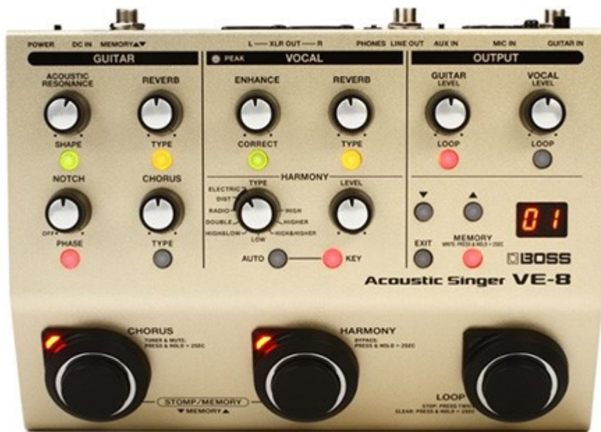
Figure 5: Intended for singer/songwriter-type live acts, the BOSS VE-8 does pitch correction and harmony generation for voice but also includes controls and processing for acoustic guitar.
