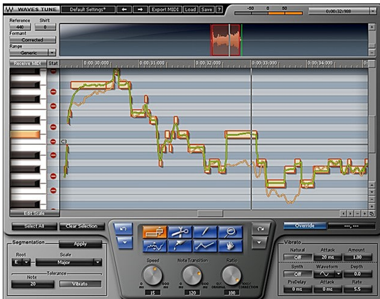
Figure 3: Waves Tune is being used to flatten the vocal pitch and give more of the hip-hop pitch correction sound, along with synthetic vibrato.
