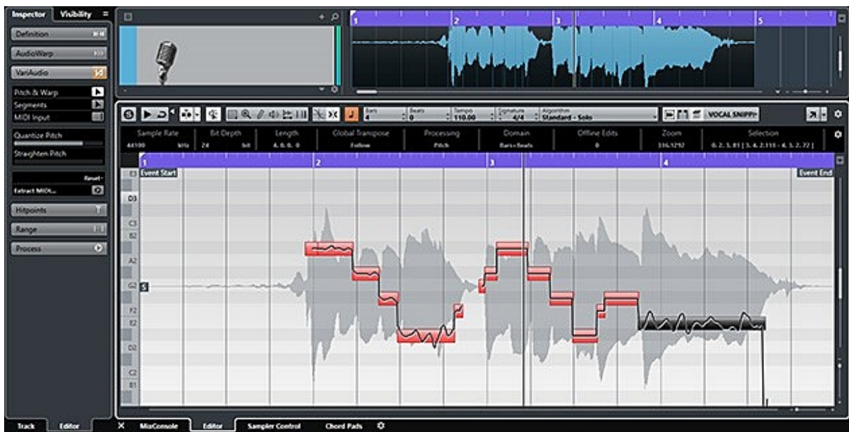
Figure 4: Cubase VariAudio makes it easy to quantize and flatten (or emphasize) pitch variations. In this example, the notes in measure 3 have been flattened to give the “Believe” pitch correction effect.
