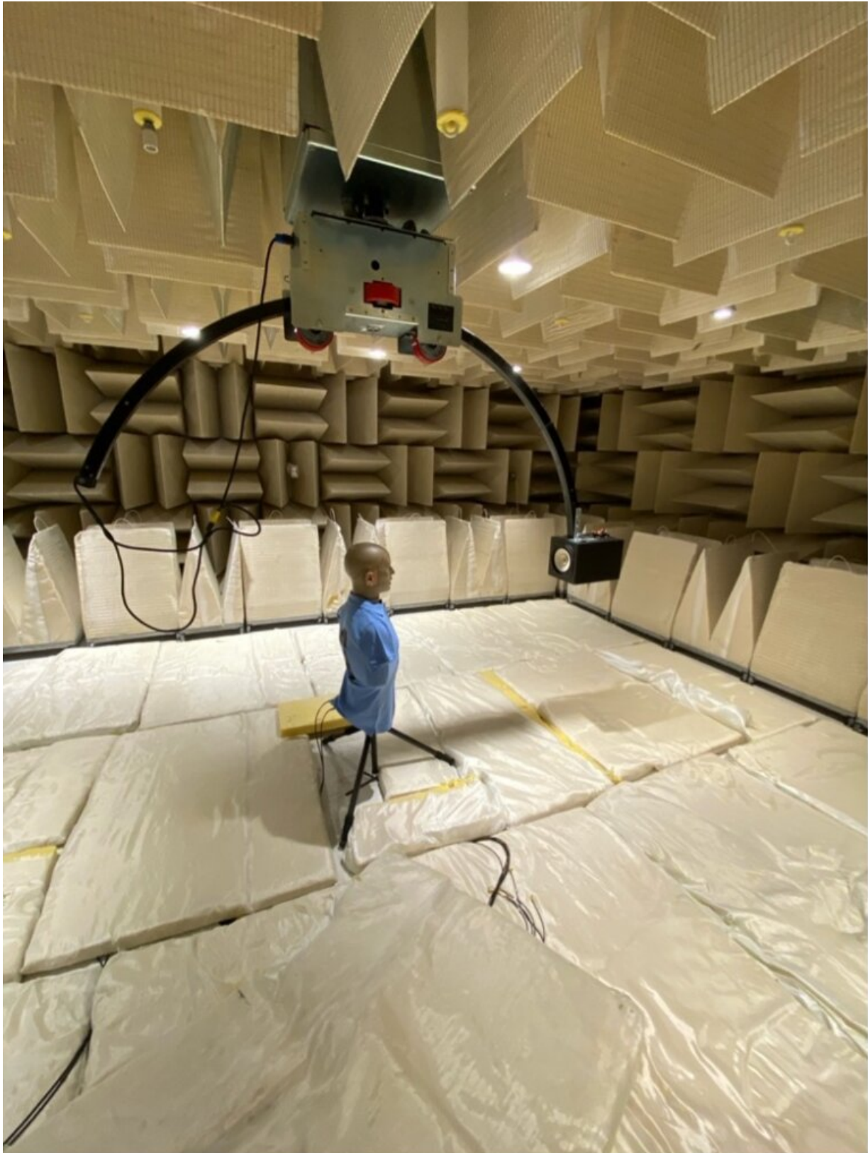
Figure 3: Experimental setup used to measure acoustic performances of DTC devices such as acoustic transparency and noise reduction.
