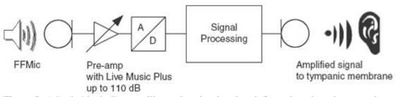
Figure 2. A basic block diagram illustrating the signal path from the microphone, to the compressor, to A/D converter, to amplifier, and finally to the receiver.
