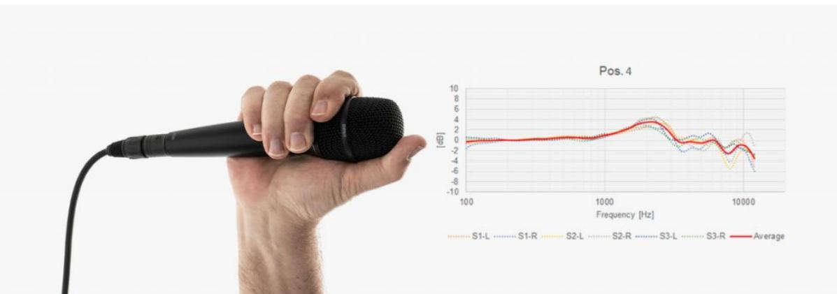
cal position – the hand covers half the grid and the thumb is laid over the top. The major resonance is found at around 2 kHz (low Q) and again above 6 kHz.
