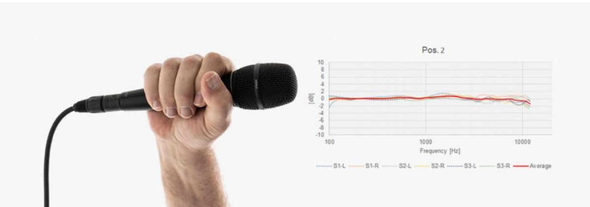
Microphone at the top of the handle, just beneath the mic head, gives the ripple a somewhat higher amplitude compared to the low position. It may be audible, however still only to a minor degree.
