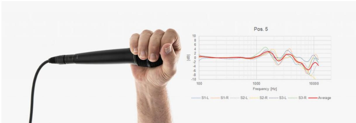
The hand surrounds the microphone head, which makes the resonances more distinct. The major resonance is found at around 2 kHz; however, at around 3-4 kHz resonances are also created due to the cavity in front of the microphone.
