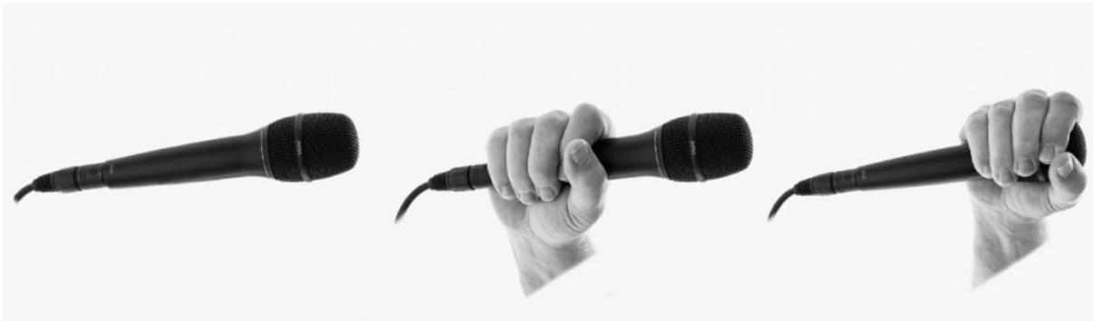
However, the hand is not the only influencing obstacle; the singer's head is also very close to the microphone. Both the hands and head affect the sound field. The microphone design, coupled with the way it is used, determines how much the sound of the microphone will be influenced.
