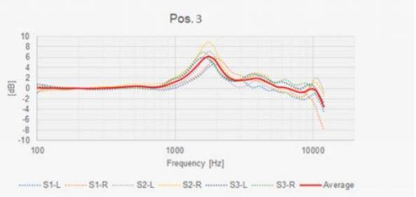
the index finger and the thumb flush with the front of the microphone creates resonances. The main resonance is, in one case, in the range of +9 dB @ 1.8-2.2 kHz. Another resonance is found around 10 kHz. This resonance is audible (coloring the audio) and is a source of acoustic feedback in the PA system.
