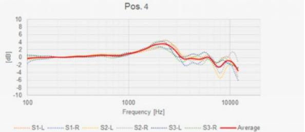
cal position – the hand covers half the grid and the thumb is laid over the top. The major resonance is found at around 2 kHz (low Q) and again above 6 kHz.
