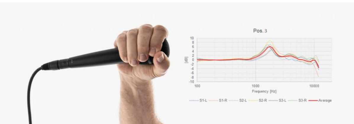
the index finger and the thumb flush with the front of the microphone creates resonances. The main resonance is, in one case, in the range of +9 dB @ 1.8-2.2 kHz. Another resonance is found around 10 kHz. This resonance is audible (coloring the audio) and is a source of acoustic feedback in the PA system.
