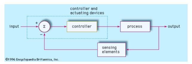
Usually, the sensors will feedback a signal that attenuates the input. This **negative feedback** will effectively maintain the process such that the final output has a stable level. If the feedback control is positive, the input to the process will increase and the output will be amplified. Ultimately, in an acoustic system, this can lead to a feedback ringing or whistling (as sometimes occurs with hearing aids).
