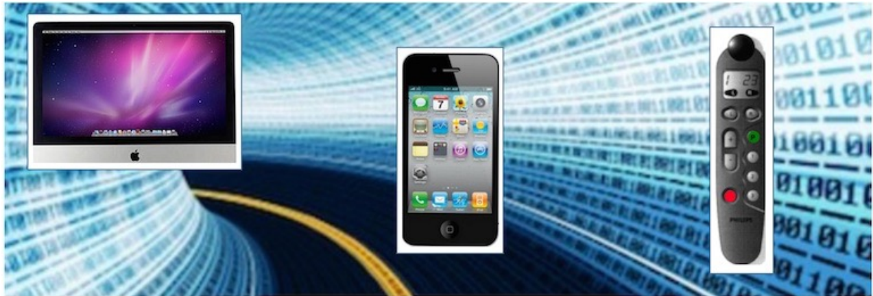
Figure 2. Remote teleprogramming (RTP) allows for hearing aid acoustical performance to be modified via the telephone from anywhere in the world. The telephone (center) is acoustically connected to the multi-programmer remote control (right). The telephone receives its DTMF signals from the primary computer program (left).
