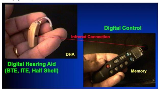
Figure 1. Hearing aid system, consisting of a hearing aid (left) and a user controlled hand-held remote multiprogrammer (right).
