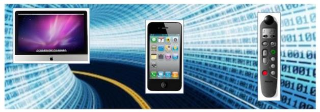
Figure 2. Remote teleprogramming (RTP) allows for hearing aid acoustical performance to be modified via the telephone from anywhere in the world. The telephone (center) is acoustically connected to the multi-programmer remote control (right). The telephone receives its DTMF signals from the primary computer program (left).
