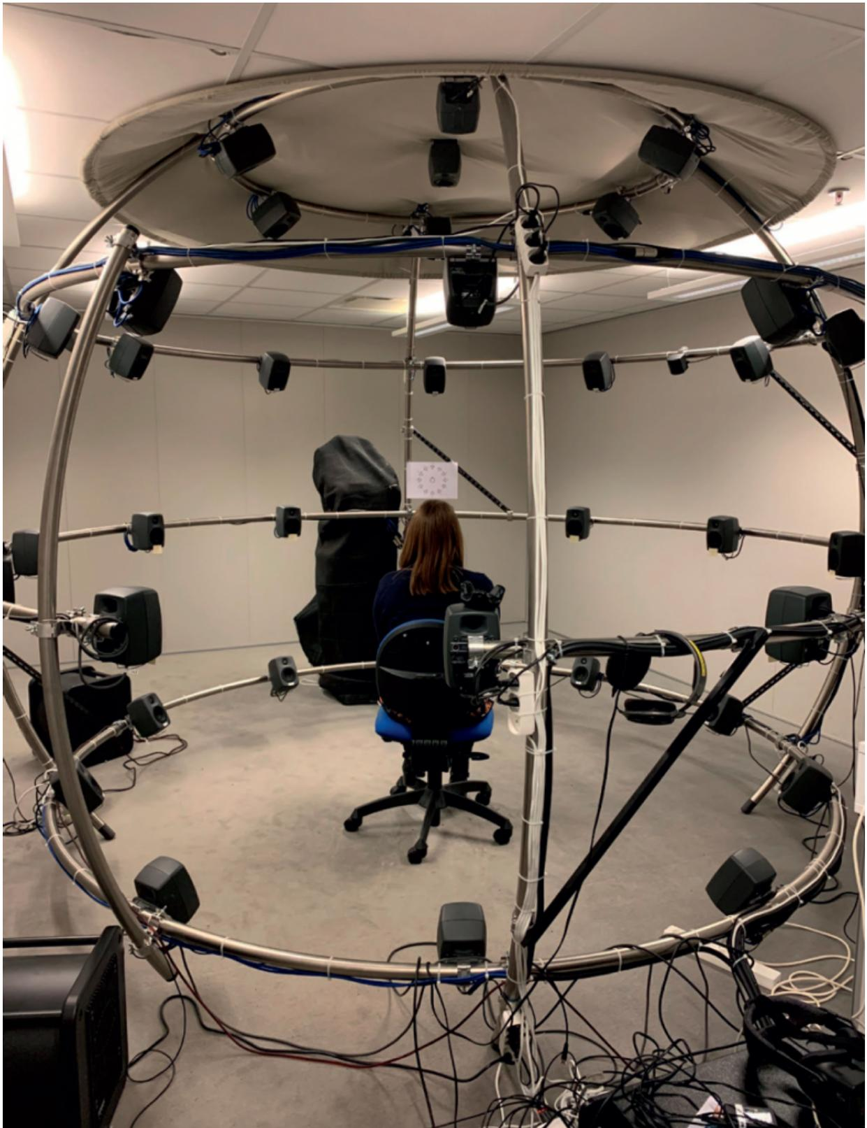
Figure 2. Test environment with 39-speaker playback array.
