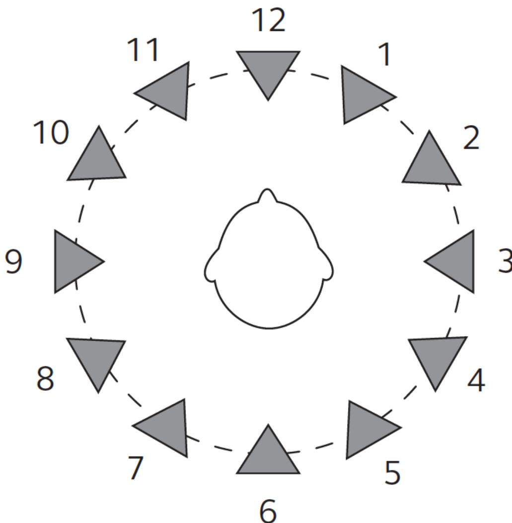
Figure 4. Sketch of the 12-loudspeaker array used for localisation testing.
