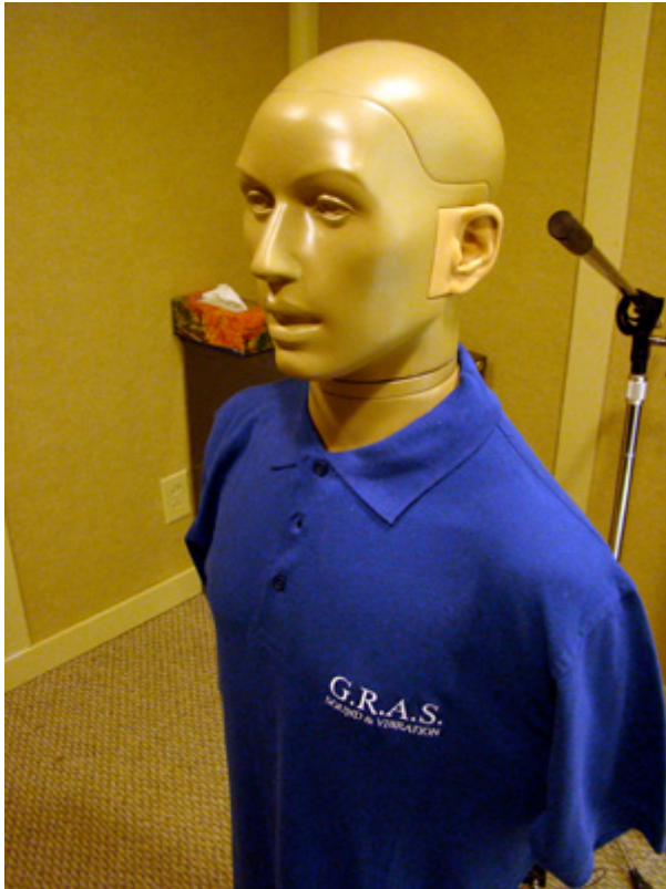
Figure 1. The Knowles Electronics Manikin for Acoustic Research (KEMAR) is a permanent lab resident. He often lends his ears to make recordings of hearing aid processing at the ear drum.
