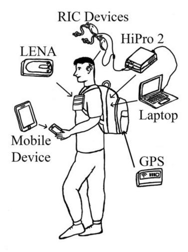
Figure 1. Illustration of user-worn devices.
