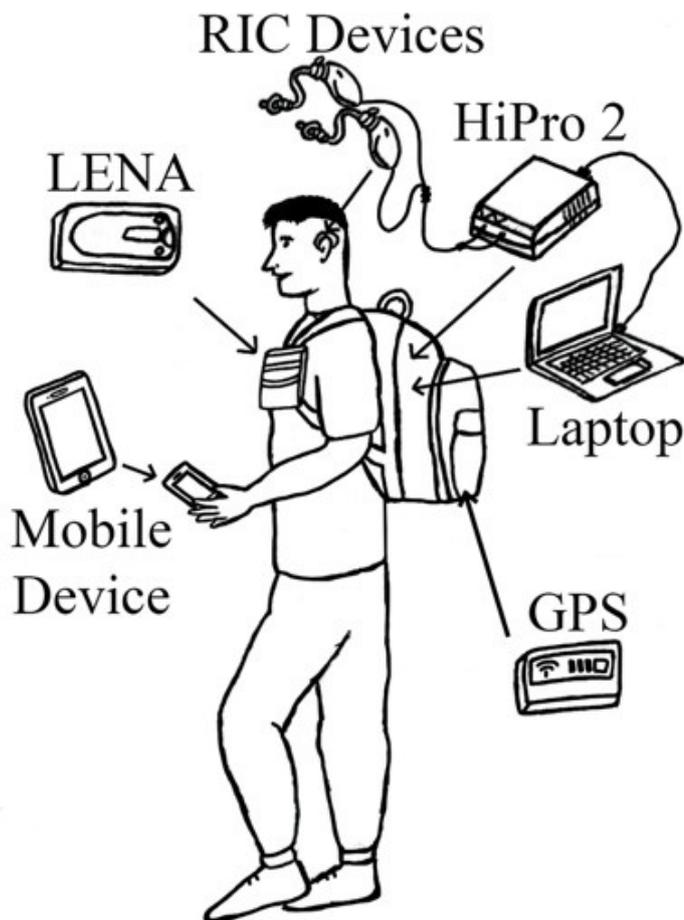
Figure 1. Illustration of user-worn devices.
